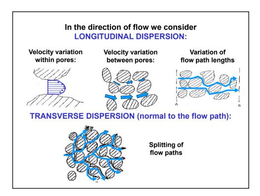
These physical mixing processes are combined and referred to as "Mechanical Dispersion" Mechanical dispersion is related to average pore velocity by dispersivity (α)
