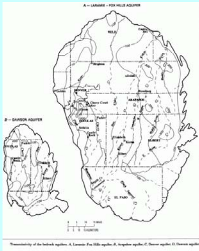
Transmissivity of the bedrock aquifers. A, Laraine-Fox Hills aquifer; B, Arapahoe aquifer; C, Denver aquifer; D, Denver aquifer.
