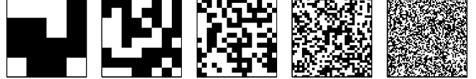
Fig. 2. Size 64 \times 64 noiselet basis functions used for collecting random measurements at a sequence of 5 scales. Each measurement is the inner product of one such function with the image of interest.
