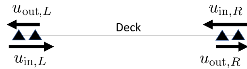
Figure 8. Decomposition of the wavefield propagating through a deck into incoming and outgoing waves at two locations of the deck. Triangles indicate the location of accelerometers. The color version of this figure is available only in the electronic edition.
