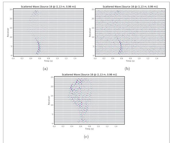
**Figure 8.** (a) A noise-free shot gather showing the recorded scattered pressure field  $p_s$ . (b) The same shot gather in (a) superimposed with uniformly distributed noise lying in the same frequency band as  $p_s$ . The SNR = 0.3. Note that only the primary scattered wave is visible at this noise level. (c) A common shot gather showing the scattered pressure field  $p_s$  for the case in which only the mass density  $\rho$  varies as shown in the right panel of figure 7.
