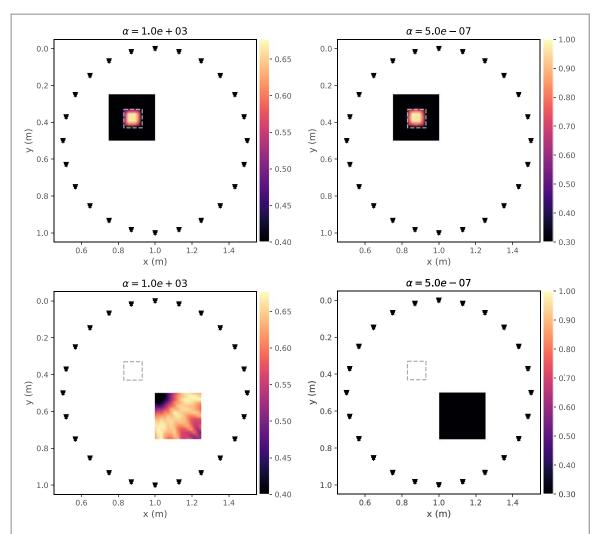
**Figure 6.** Reconstructions of the box-shaped anomaly using (left column) Lippmann-Schwinger inversion and (right column) the linear sampling method. *Top row:* the imaging domain contains the scatterer. *Bottom row:* the imaging domain does not contain the scatterer. Images in the bottom row are plotted on the same scale as the corresponding image in the top row. The value of the regularization parameter  $\alpha$  is indicated above each plot.
