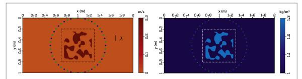
**Figure 7.** Models of the acoustic velocity (left) and mass density (right) for the random inclusions. Sources are indicated by blue dots and receivers by green dots. The dashed line indicates the imaging domain. The dominant wavelength of the Ricker pulse is shown for scale.
