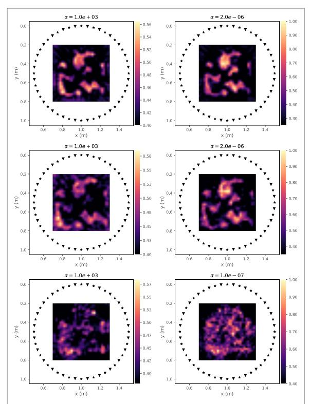
Figure 9. Reconstructions of the random inclusions using (left) Lippmann-Schwinger inversion and (right) the linear sampling method. *Top row:* reconstructions obtained using the correct background model and noise-free data. *Middle row:* reconstructions obtained using an erroneous background velocity model and noisy data. *Bottom row:* reconstructions obtained for the case in which only the mass density varies. The value of the regularization parameter  $\alpha$  is indicated above each plot.
