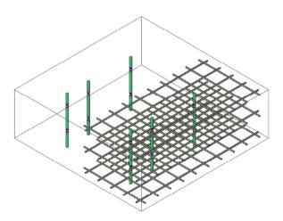
Figure 7.1: Schematic of the 3D concrete block for time-lapse monitoring
