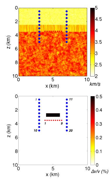
Figure 6.2: Numerical model for time-lapse inversion of localized velocity change with the used sources (red circles) and receivers (blue circles). Top: the reference velocity (scattering) model with the source-receiver setup and Bottom: the true localized velocity change with the source-receiver setup.
