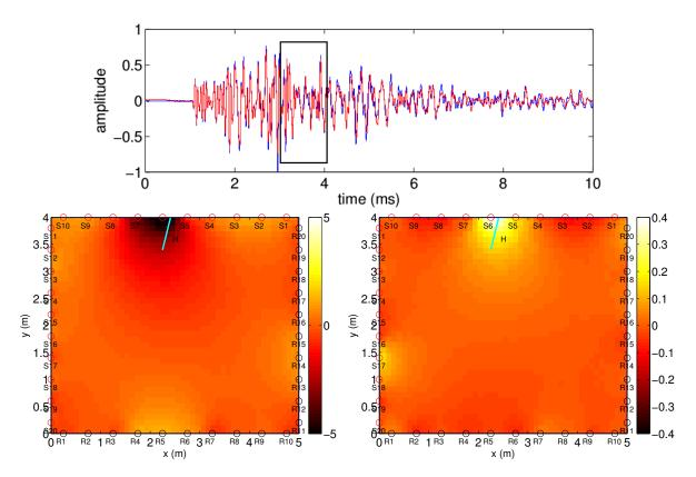
Figure 7.15: Inverted change due to localized temperature change due to a heating cartridge at H (Figure Figure 7.5 (Bottom)) using the travel-time changes and decorrelation estimated at the coda time window (black rectangle) in Top inset. In the Bottom inset: (left) the inverted relative velocity change (in percentage) using estimated travel-time changes and (right) the inverted change in the scattering cross-section (in  $m^2$ ) using estimated decorrelation.
