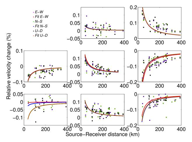
Figure 8.7: The relative velocity change estimated for each of the time-lapse periods as a function of source-receiver distance. Power law fitting of the estimated velocity changes in Utah Wasatch fault region. Fit E-W, N-S, and U-D are the fitting solutions for the estimated velocity changes of E-W, N-S, and U-D components, respectively.
