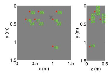
Figure 7.2: Outline of the 3D concrete block with the locations of the used transducers. The transducers are embedded within the concrete block. The transducer locations are the projection along the z-axis (left) and along the x-axis (right).
