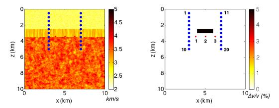
Figure 3.8: Numerical model for time-lapse localized velocity change. The reference velocity (scattering) model (a) with the source-receiver setup, and the exact localized velocity change (b) with the source-receiver setup.
