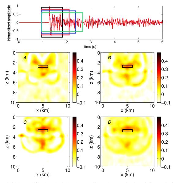
Figure 6.8: Inverted fractional velocity change using various coda time windows. Top inset: a typical recorded coda signal with time windows use to invert the velocity changes. Inverted velocity change in A: with black time window, B: with red time window, C: with blue time window, and D. with green time window. The black box shows the extent of the velocity change.
