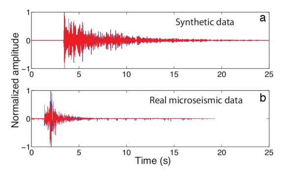
Figure 3.1: Synthetic time-lapse signals (a) and recorded microseismic time lapse signals (b). The blue curve is the baseline signal and the red curve is the time-lapse signal.
