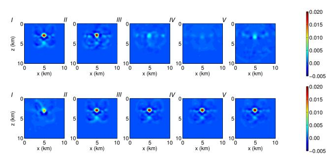
Figure 6.6: The point spread function  $\mathbf{p}^i$  for the inverted model at [x, z] = [5, 3] km using the Top: Category 1 and Bottom: Category 2 time-windows. The point spread function  $\mathbf{p}^i$  uses time-windows: I (black window), II (red window), III (blue window), IV (green window), and V (yellow window) in Figure 6.5.
