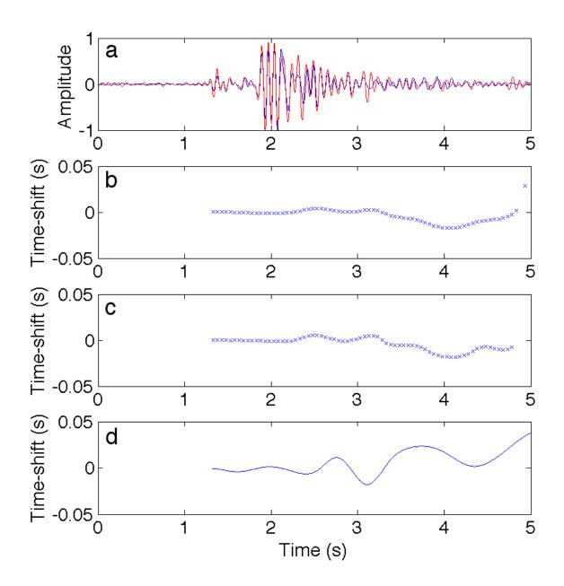
Figure 3.6: Time shifts computed from the 5-15Hz bandpassed time-lapse microseismic signals (a) using windowed cross-correlation (b), the windowed stretching method (c), and SDTW (d).
