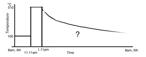
Figure 7.8: Temperature history of the time-lapse heating experiment. The question mark indicates that the temperature curve between 1:11pm ( $4^{th}$  of April) and 8am ( $5^{th}$  of April) is unknown.
