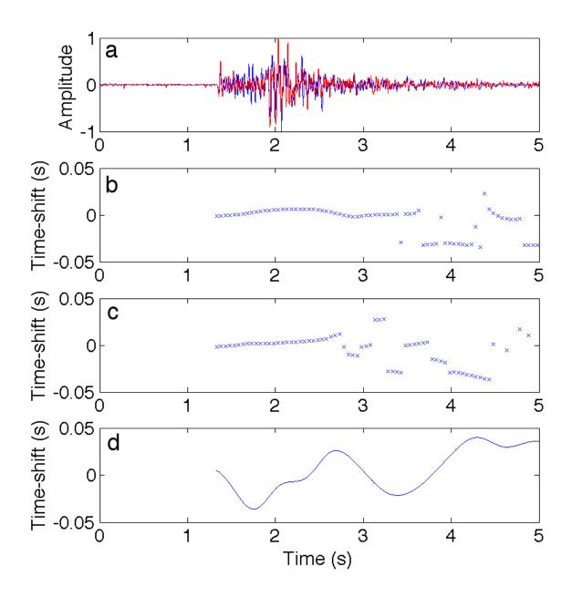
Figure 3.5: Time shifts computed from the unfiltered time-lapse microseismic signals (a) using windowed cross-correlation (b), the windowed stretching method (c), and SDTW (d).
