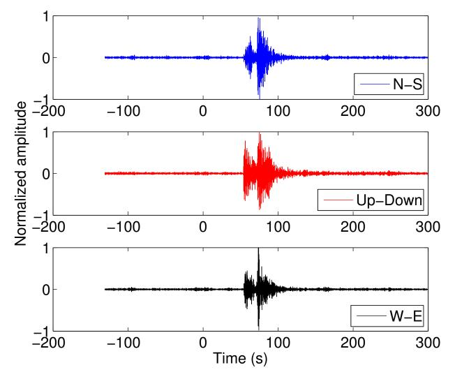
Figure 8.3: Typical recordings of the blast events bandpass filtered between 1-5 Hz. The three components, N-S (blue), Up-Down (U-D) (red) and the E-W (black) are all used in the time-lapse analysis. The black rectangle gives the coda section of the blast signal.
