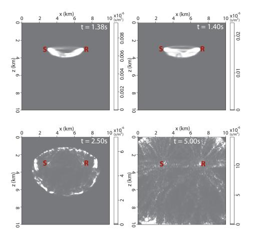
Figure 4.13: Temporal and spatial evolution of the sensitivity kernel (numerical solution) in a reservoir with shale-like velocity perturbation.
