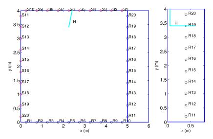
Figure 7.5: The pictorial (Top) and the schematics (bottom) of the concrete block use for the time-lapse temperature monitoring experiment. The cyan line gives the heating cartridge probe.
