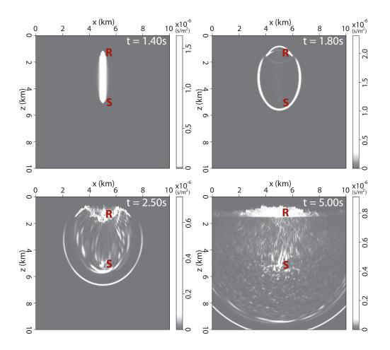
Figure 4.15: Temporal and spatial evolution of the sensitivity kernel (numerical solution) showing topography-induced scattering using vertical source-receiver line.
