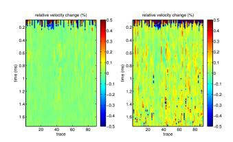
Figure 7.11: Record of the estimated time-lapse relative velocity change in % due to a load jump from 5 kN to 10 kN (left) and a load jump from 5 kN to 15 kN (right). The record contains 90 traces (due to 10 pairs of sensors with no trace for the same sensor combination). The records are arranged according to the source sensor records.
