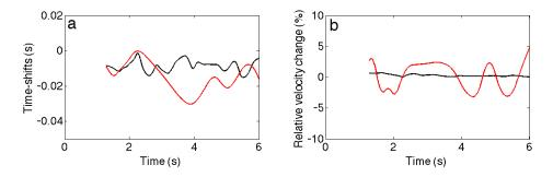
Figure 3.9: A comparison of the estimated time shifts (a) and relative velocity changes (b) using stretching method (black) and smooth dynamic warping (red). These timeshifts and velocity changes are estimated using the time-lapse signals for Source 2 and Receiver 3 pair shown in Figure 3.8.
