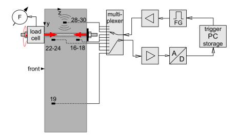
Figure 7.3: The electrical and mechanical setup of the stress loading experiment.
