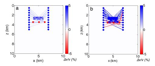
Figure 3.11: Distribution of the relative velocity changes between time-lapse signals computed using the stretching method (a) and SDTW (b) among source-receiver pairs. The velocity changes are estimated using the early part of the time-lapse coda. Blue circles are the receivers while the red circles are the sources. The blue rectangle gives the localized time-lapse velocity change of 5%. The colored lines indicate the magnitude of the estimated relative velocity changes.
