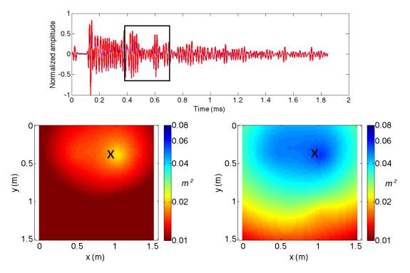
Figure 7.14: Inverted change due to stress loading from 5 kN to 10 kN (left) and from 5 kN to 15 kN (right) at X. Top inset: Time-lapse coda showing the time-window used for the inversion.
