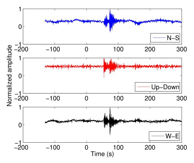
Figure 8.2: Example recording of typical blast events. Event 09/10/2007 recorded at station L13A. The three components, N-S (blue), Up-Down (U-D) (red) and the E-W (black) are all used in the time-lapse analysis.
