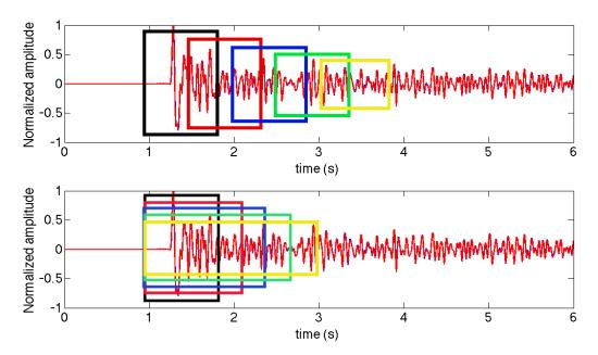
Figure 6.5: The coda time windows use for resolution analysis for the time-lapse imaging. Top: The used time windows for Category 1 resolution analysis and Bottom: The used time windows for Category 2 resolution analysis.
