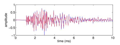
Figure 7.7: Typical coda signal recorded by sensor R5 due to a source at sensor S1 from the temperature experiment.
