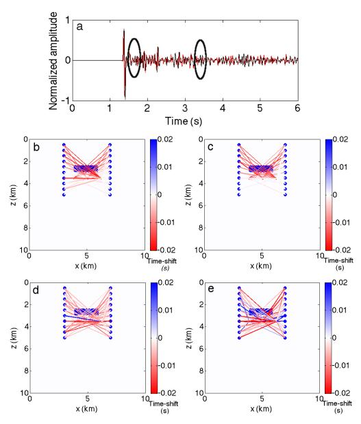
Figure 3.10: The early (near t = 1.6 s) and late (near t = 3.4 s) coda of the time-lapse signals (a) are highlighted. Time shifts from the early coda are computed using the stretching method (b) and SDTW (c), and time shifts in the late coda are also computed using the stretching method (d) and SDTW (e). The colored lines indicate the magnitude of the estimated traveltime changes.
