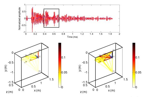
Figure 7.12: Time-lapse decorrelation due to stress loading from 5 kN to 10 kN (left) and from 5 kN to 15 kN (right) at X. The colored lines between two sensors are the estimated average decorrelation between the time lapse signals using equation 7.3 for the time-window in time-lapse coda (top). The decorrelations for each sensor pairs are not restricted to the connecting colored lines.
