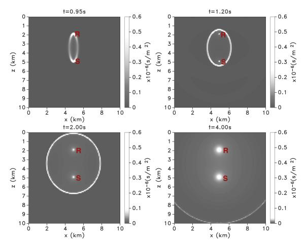
Figure 4.3: Temporal and spatial evolution of the sensitivity kernel using the radiative transfer model.
