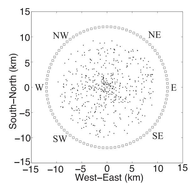
Figure 2.2: The experiment geometry of the numerical simulation. The receivers (squares) are surrounding the point scatterers (black dots). The source is positioned in the origin (cross). All perturbations of the source location is done from this position. The stations marked (NW, NE, E, SE, and SW) are used in the presentation of results in Figure 2.7 and Figure 2.8.
