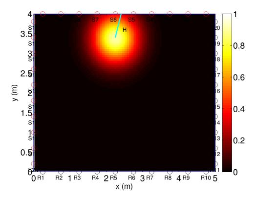
Figure 7.9: Normalized temperature distribution across the heated concrete medium at the end of the temperature history in Figure 7.8 using equation 7.10. The cyan line is the heating cartridge probe.
