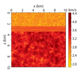
Figure 4.11: Velocity model with a shale-like reservoir.
