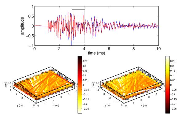
Figure 7.13: Time-lapse fractional velocity change (%) and decorrelation due to temperature change within the concrete block. The colored lines between two sensors are the estimated changes (fractional velocity change (left) and decorrelation (left)) between the time lapse signals for the time-window in time-lapse coda (top). The changes for each sensor pairs are not restricted to the connecting colored lines.
