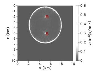
Figure 6.1: Sensitivity kernel  $K(\mathbf{s}, \mathbf{x}_{\mathbf{o}}, \mathbf{r}, t)$  for the source-receiver pair (S-R) within a statistical homogeneous scattering velocity model.
