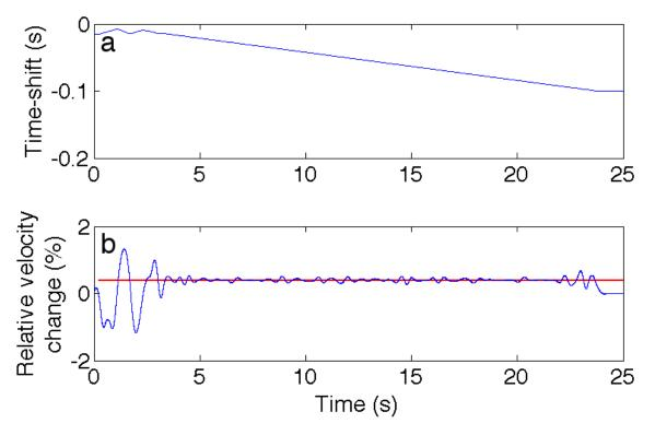
Figure 3.4: Time shifts and relative velocity changes estimated via SDTW. The time shifts (a) and the relative velocity changes (b) are computed from the synthetic time-lapse signals shown in Figure 3.1a. We compare the exact velocity change (red) to the estimated relative velocity changes (blue) (b).
