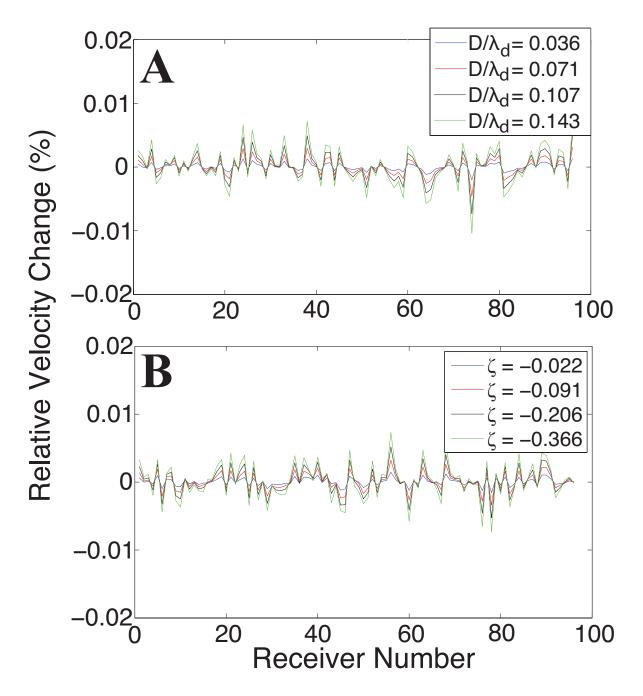
Figure 2.6: Estimated relative velocity change due to perturbation in the source location and the source radiation. A. The estimated velocity change for perturbed source location (divided by the dominant wavelength; inset in the top right) and B. The estimated velocity change caused by changes in source radiation angles (inset in the top right). The value of  $\zeta$ is given by equation 2.15. The receiver numbers are counted counter-clockwise from the W station in Figure 2.2.
