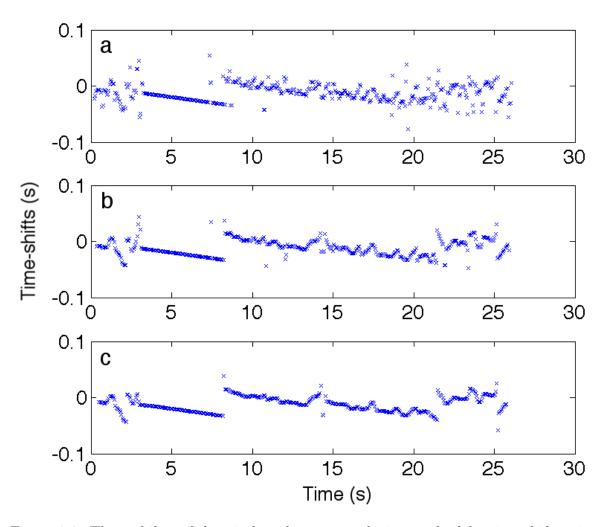
Figure 3.2: The stability of the windowed cross-correlation method for time shift estimation. The time shifts are estimated within time windows whose widths  $2t_w$  are relative to the dominant period T of the signal:  $2t_w = 37.5T$  (a),  $2t_w = 75T$  (b), and  $2t_w = 112.5T$  (c), where T = 0.033 s.
