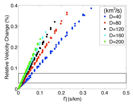
Figure 8.10: Dependence of the estimated velocity change on the dimensionless parameter  $\eta$ . The definition of  $\eta$  is given in equation 6. The black rectangle corresponds to the range of velocity changes estimated with station J13.
