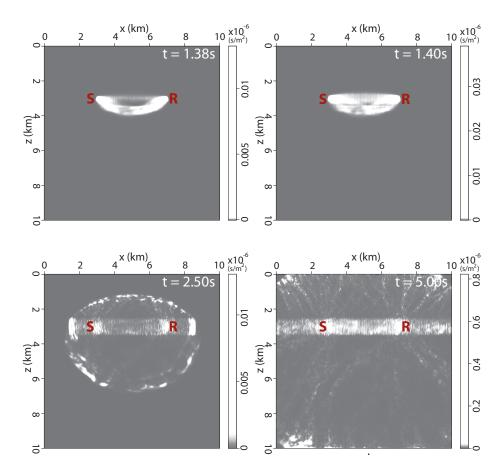
Figure 4.10: Temporal and spatial evolution of the sensitivity kernel (numerical solution) in a reservoir with vertical-fractured-like velocity perturbation with a receiver within the reservoir.
