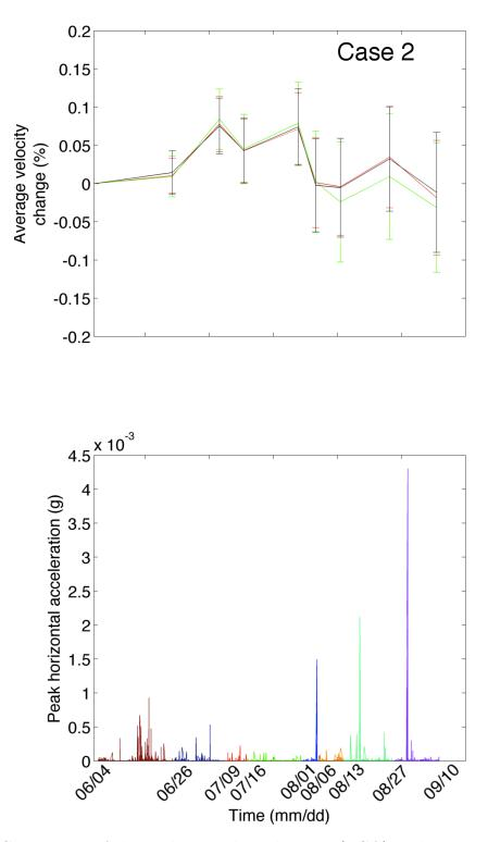
Figure 8.13: Comparison of the peak ground acceleration (PGA) with average relative velocity change estimated in Case 2. The PGA values are estimated from the local seismicity (M > -0.36) that occurred during the monitored time-lapse period. The PGA values are estimated using relationship between PGA and the magnitude of an earthquake Chiou et al. [17].
