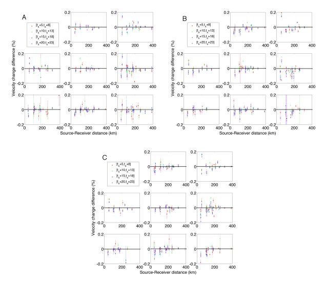
Figure 8.8: Estimated velocity change difference  $\Delta_T$  for each time-lapse period. The plots show the estimated velocity change difference  $\Delta_T$  versus the source-receiver distance for the A: N-S component, B: Up-Down (U-D) component, and C: N-S component.
