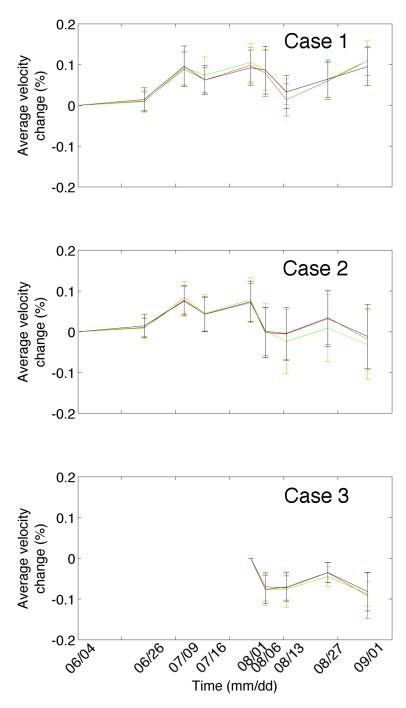
Figure 8.5: The cumulative relative velocity changes expressed in percentages for N-S (red), Up-Down (U-D) (green) and the E-W (black) components. Here the average is computed using all the stations in the USArray displayed in Figure 8.1. Missing first five estimates in Case 3 is because only signals from August 1 is processed in Case 3.
