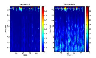
Figure 7.10: Record of the estimated time-lapse decorrelation due to a load jump from 5 kN to 10 kN (left) and a load jump from 5 kN to 15 kN (right). The record contains 90 traces (due to 10 pairs of sensors with no trace for the same sensor combination). The records are arranged according to the source sensor records.
