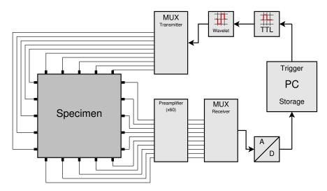
Figure 7.6: The electrical and mechanical setup of the stress loading experiment.
