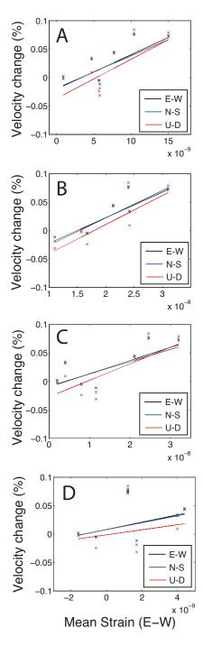
Figure 8.12: Linear regression between the E-W strain derived from E-W GPS detrended displacement and the individual components of average velocity change (E-W, N-S, and vertical components). The linear regression is computed using A, all the available GPS displacement, B, only the Basin and Range GPS displacements, C, only the Wasatch fault displacements, and D, only the Snake River Plain GPS displacements.
