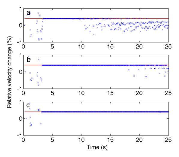
Figure 3.3: The stability of the windowed stretching method for relative velocity change estimation. The relative velocity changes are estimated within time windows whose widths are relative to the dominant period T of the signal: 37.5T (a), 75T (b), and 112.5T (c), where T = 0.033 s. The red line shows the exact relative velocity change.
