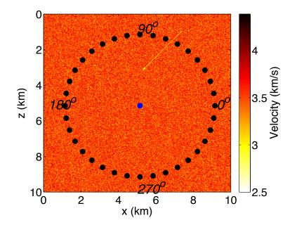
Figure 6.4: The model geometry use for data averaging test. A Gaussian velocity change is centered at location [x, z] = [3, 5] km within a statistically homogeneous velocity model. The data averaging test used a ring of receivers (black dots) and s source (blue dot) located at [x, z] = [5, 5] km. The azimuth of the receivers is specified by the degrees. The yellow arrow points to the location of the velocity change.
