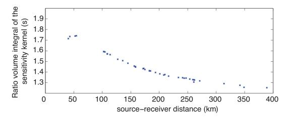
Figure 8.14: Increased sensitivity due to the presence of Moho interface at depth 25km based on the ratio of the volume integral of the sensitivity kernel with and without the Moho interface.
