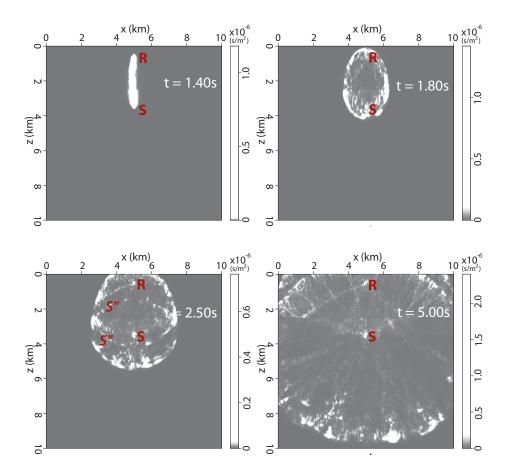
Figure 4.9: Temporal and spatial evolution of the sensitivity kernel (numerical solution) in a reservoir with vertical-fractured-like velocity perturbation with a near-surface receiver. S'' corresponds to the reflected scattered phase.
