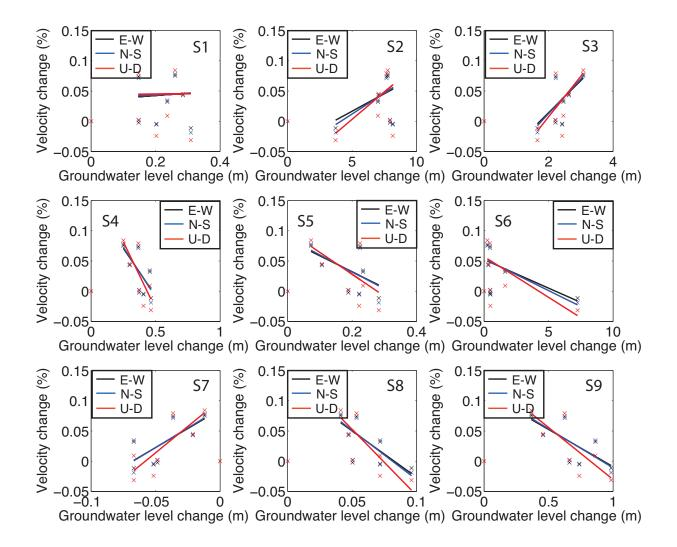
Figure 8.11: Correlation of average velocity change with groundwater level change measured in meters (positive meters mean deepening of the groundwater level). Each plot shows the fit of the average velocity changes from the three signal components. S1 to S9 are the names of the groundwater wells.
