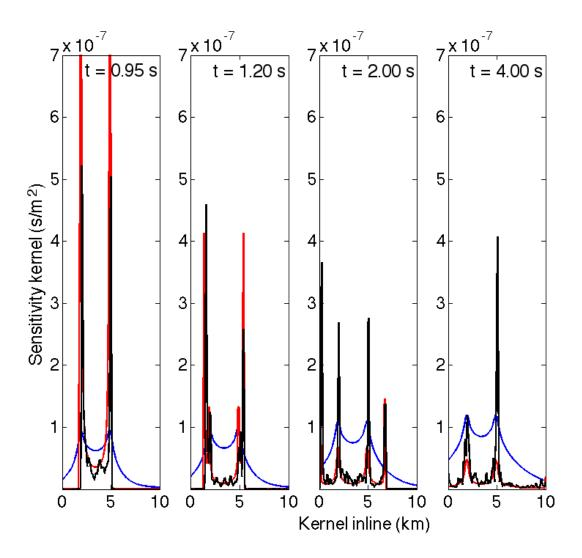
Figure 4.5: Comparison between numerical sensitivity kernel (black line) and diffusion- (blue line) and radiative transfer- (red line) based kernel along the source- (at  $2 \ km$ ) receiver- (at  $5 \ km$ ) line.
