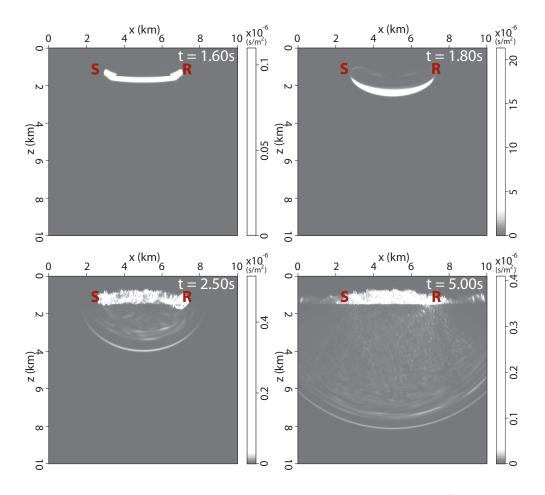
Figure 4.16: Temporal and spatial evolution of the sensitivity kernel (numerical solution) showing topography-induced scattering using horizontal source-receiver line.
