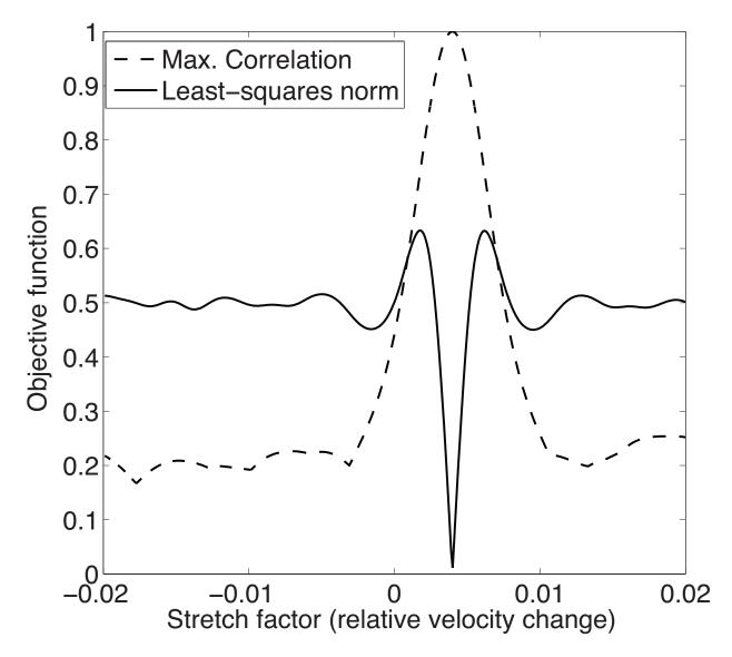
Figure 2.4: The objective function  $R(\epsilon)$  (solid line) as a function of the stretch factor  $\epsilon$ . The objective function is minimum for  $\epsilon = 0.4\%$ , which corresponds to the time-lapse velocity change. The corresponding maximum correlation of the stretch factors is given by the dash lines.
