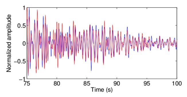
Figure 8.4: A typical time-lapse coda of the 1-5 Hz filtered recorded blast events for the Up-Down (U-D) component.
