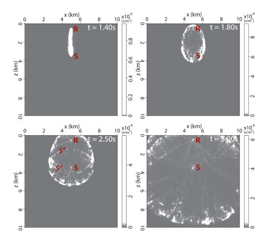
Figure 4.12: Temporal and spatial evolution of the sensitivity kernel (numerical solution) in a reservoir with shale-like velocity perturbation. S'' corresponds to the reflected scattered phase.
