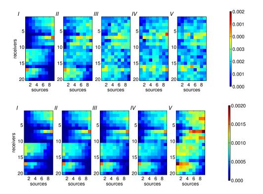
Figure 6.7: Data spread function for the inverted model using the Top: Category 1 timewindows and Bottom: Category 2 time-windows. Each value is an estimated fractional velocity change for a given source-receiver pair.
