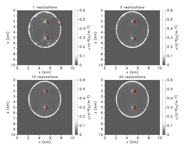
Figure 4.6: Compassion of the kernel at  $t = 2.0 \ s$  using a number of scattering model realizations
