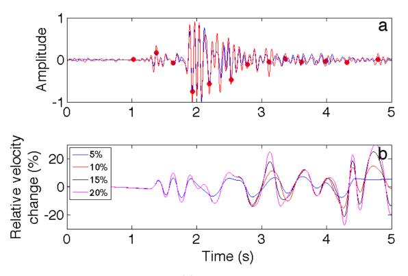
Figure 3.7: Relative velocity changes (b) computed from the 5-15Hz bandpassed time-lapse microseismic signals (a) using SDTW and multiple bounds on du/dt. Time shifts are sampled on an amplitude-aligned coarse grid (red points) (a).
