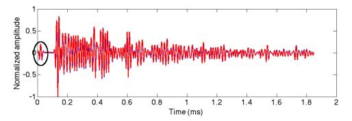
Figure 7.4: Typical time-lapse coda signals recorded at transducer 17 due to a source at transducer 16 from the stress loading experiment. The black ellipse indicate the electrical signal use to book-keep the source unset time.
