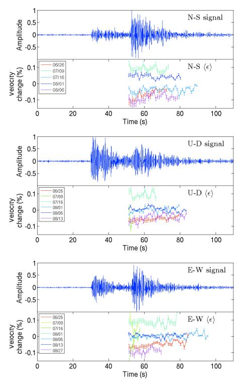
Figure 8.9: Estimated velocity change  $\langle \epsilon \rangle$  versus time in the coda for each time-lapse period using the N-S component (top), the Up-Down (U-D) component (middle), and the E-W component (bottom).
