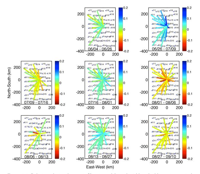
Figure 8.6: Relative velocity changes in % estimated from the 8 blast doublets using vertical component of the stations. The blue points are the surface stations. The source location is the point where all the colored lines meet. The color lines are the estimated percentage velocity changes for each source-receiver pair.
