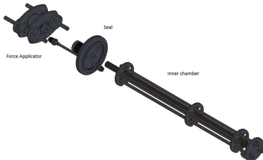
Figure 2: Multi-Mode Force & Field Assisted Sintering Device
