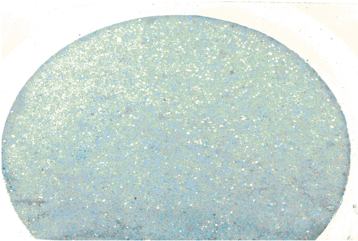
FIG. 4.8. Tubb-B carbonate: Optical thin section. Blue colored areas are the pore spaces.
