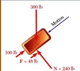
• If maximum friction force is less than friction force required for equilibrium, block will slide. Calculate kinetic-friction force.
