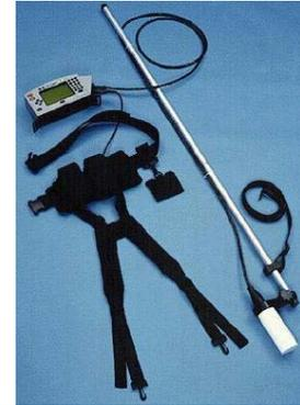
Figure 4.D.1: Geometrics G-858/G Cesium Magnetometer/Gradiometer setup for use in a traditional magnetic survey (photo courtesy of Geometrics website, accessed June 4, 2007)
