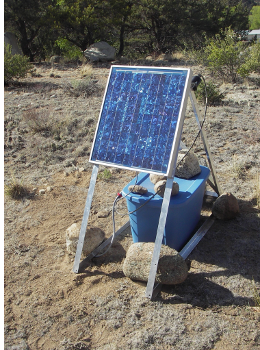
Figure 11.2: Image of a fully installed passive seismic instrument. This station is located at the Henderson Cabin in Deer Valley, CO
