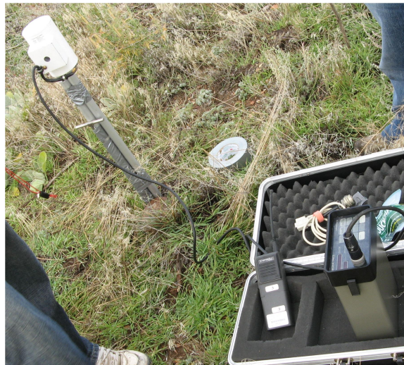
Figure 7.2: Setup of the base-station proton free-precession magnetometer
