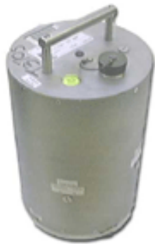
(a) Image of the Gurlan CMG-3T broadband instrument. Three of these instruments were used for the passive seismic survey.
