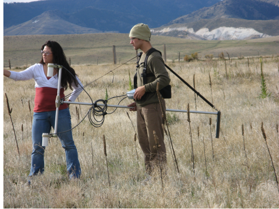
Figure 7.4: The cesium magnetometer used in the field by CSM student David Manthei
