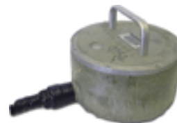
(b) Image of the Mark Products L22 short period instrument. Nine of these instruments were used for the passive seismic survey.
