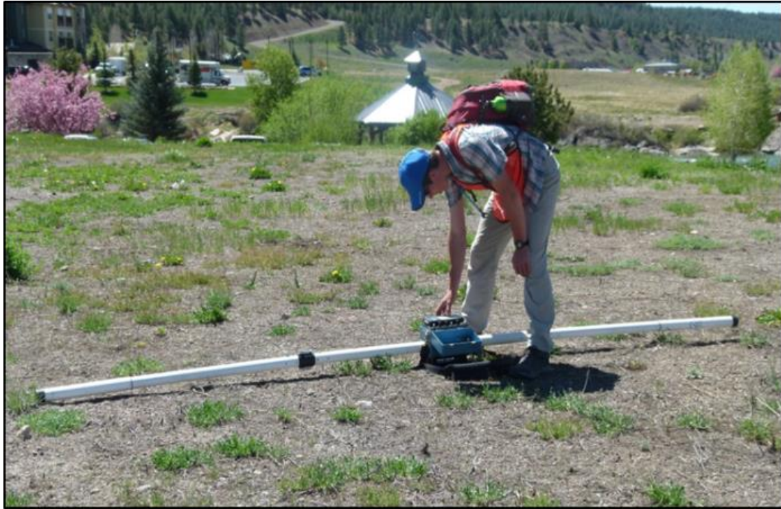
Figure E.2: A picture illustrating the EM31 during setup.
