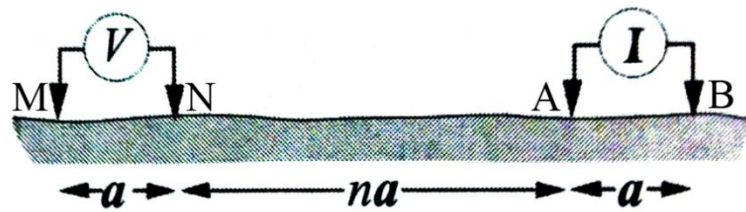
Figure F.5: Dipole-Dipole array layout [72]
