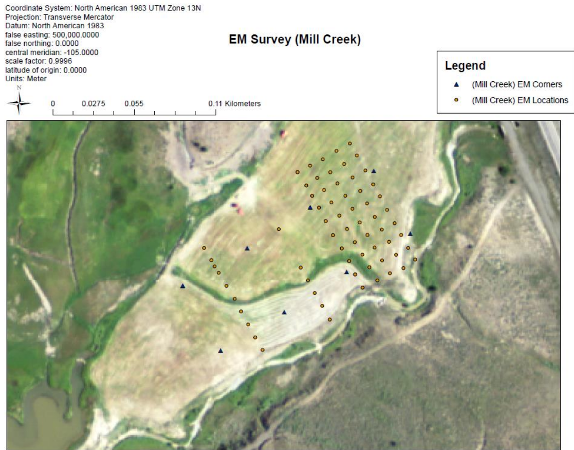
Figure 9.6: Shows the GPS locations of the EM57 grid and the EM47 lines at Mill Creek near the highway (Highway 84 is on the right side of the image).
