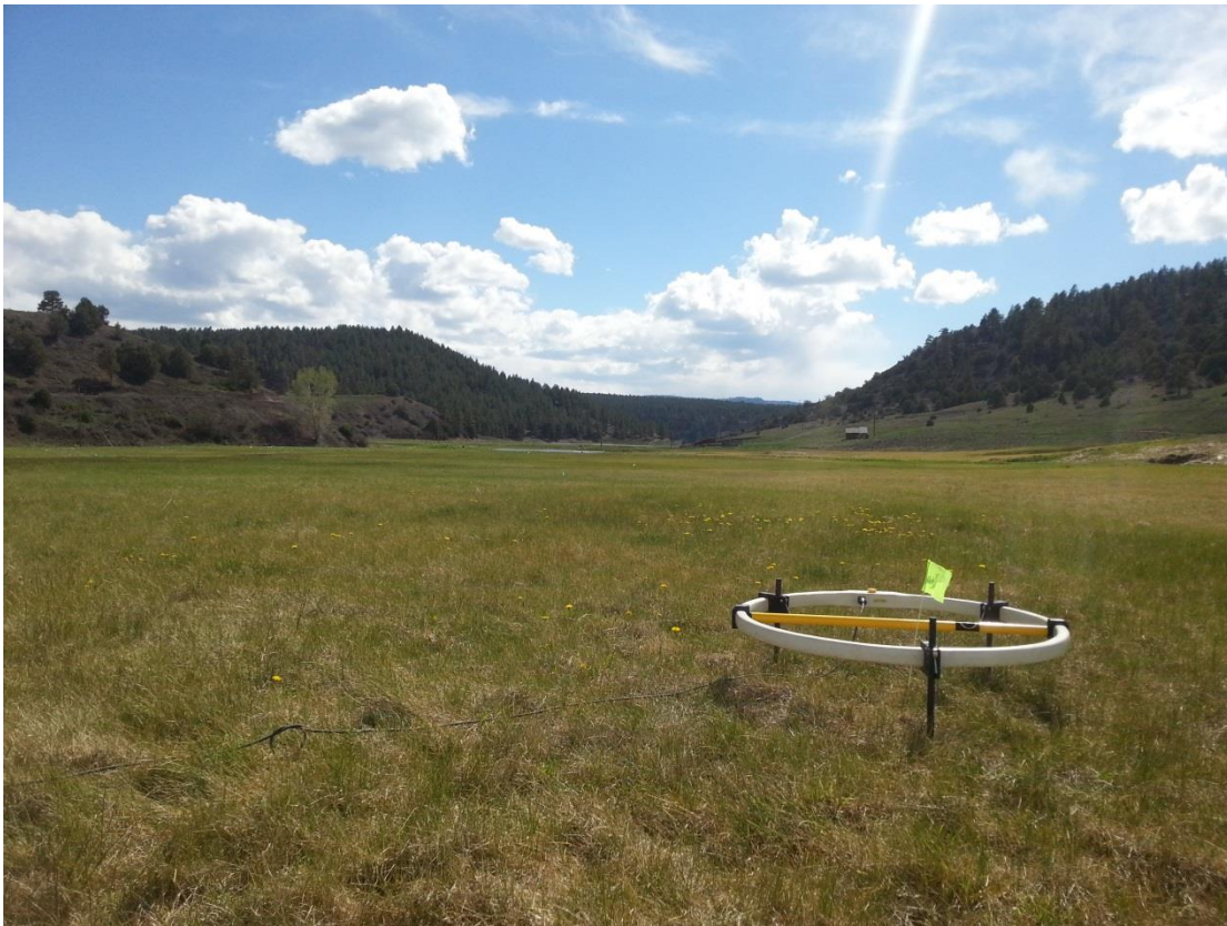
Figure E.5: An image depicting the EM57's receiver loop in action.
