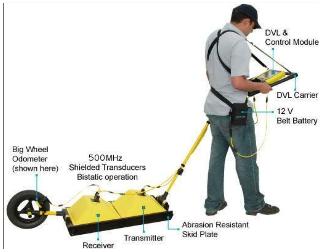
Figure 12.2: Sensors & Software pulseEKKO PRO GPR system 80
