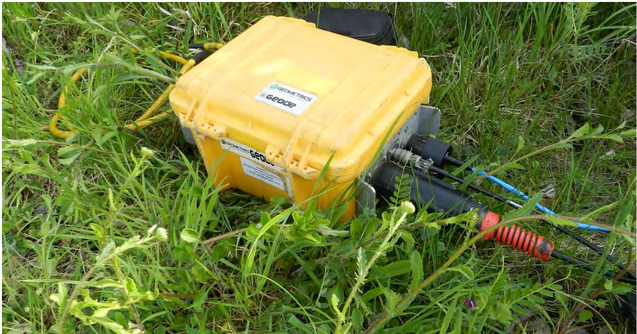
Figure 6.10: Image of the Geode seismograph used for collecting hammer seismic data. Photo courtesy of Geomatrix Earth Science LTD [41].
