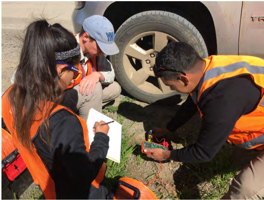
Figure 9.12: Students collecting SP data along the main line in Pagosa Springs. A multimeter is used to measure voltage between the roving electrode (shown), and the reference electrode (not shown). Data is recorded in a notebook.
