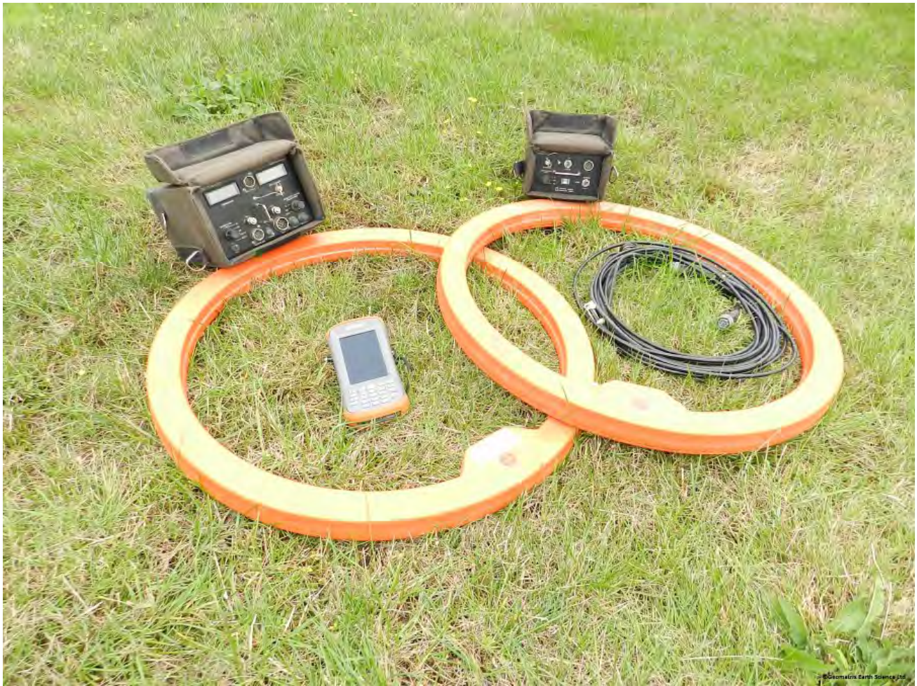
Figure 11.6: Geonics EM34 system similar to what we used (this shows an optional digital logger that our system doesn't support). The orange rings are the transmitter and receiver coils, the box leaning on the left ring is the receiver, and the smaller box on the right ring is the transmitter. [72]
