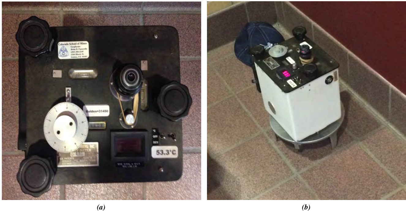
Figure 7.3: Lacoste and Romberg L&R gravimeter; (a) top view and (b) side view with leveling plate. We used the L&R gravimeter to collect gravity data at the student site north of Pagosa Springs.[45]
