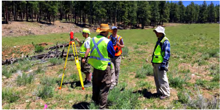
Figure 3.5: Picture of student surveyor and mentors using the total station to take points at the student site.
