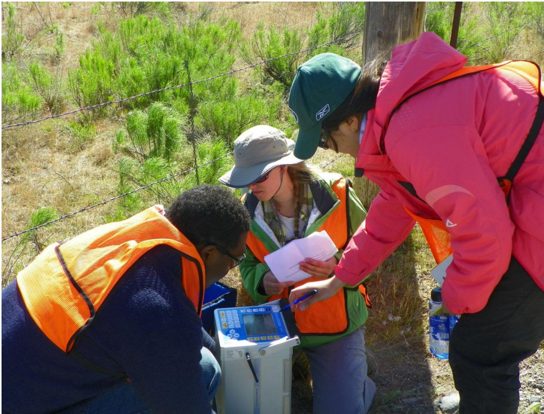
Figure 5-2 Operation of Scintrex CG5 Gravimeter
