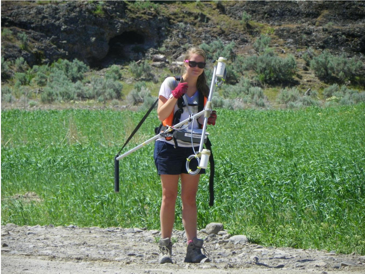
Figure 5-5 Acquisition of Magnetic Data
