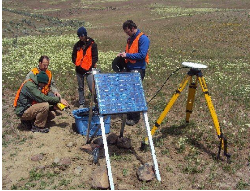
Figure 11-8 Passive Seismic Station and DGPS Base Station
