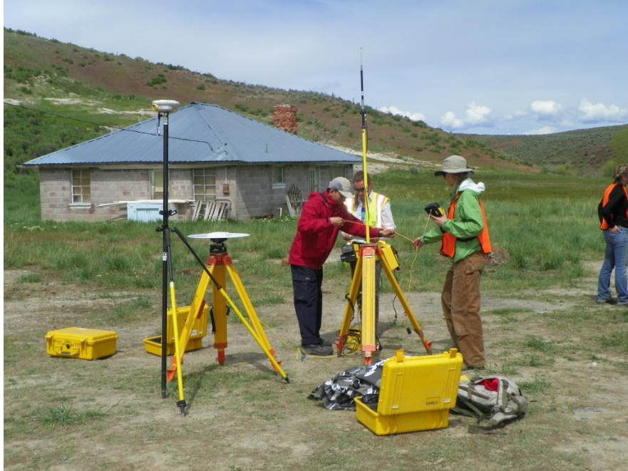
Figure 4-1 Rover and Base Station for DGPS
