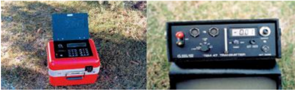
Figure 5-9 EM47 Receiver (Left) and Transmitter (Right) [Geonics Website]
