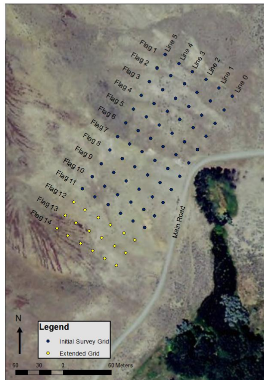
Figure 10-6 Grid Setup at the Warm Spring Site
