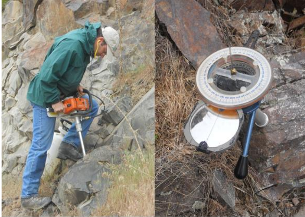
Figure 11-2 Paleomagnetic Acquisition (Left) Demonstration of the Core Drilled by Jonathon from the USGS. (Right) The compass inclinometer used to measure the in situ orientation of the core samples.
