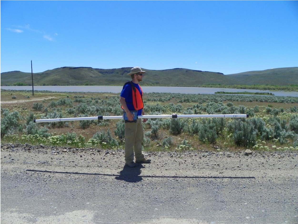
Figure 5-7 Acquisition Using the EM31 Device
