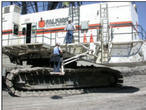
Hydraulic lift installed on a dragline improves access and eliminates climbing a vertical ladder.
