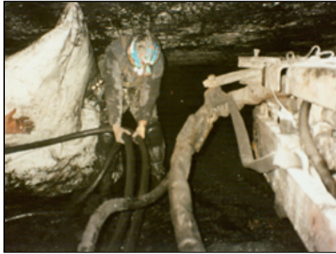
Lifting continuous miner power cable. Continuous miner cable weighs about 7 pounds per foot. Moving long sections of cable can often result in high forceful exertions. Working in restricted spaces makes the task even more difficult.
