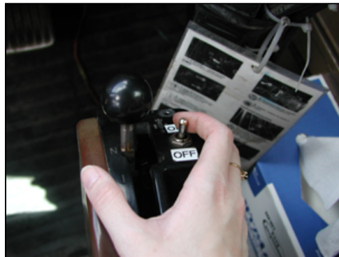
Water pump switch in a water truck was moved from the dash and relocated to the center console, which eliminates unnecessary reaching to operate the switch.
