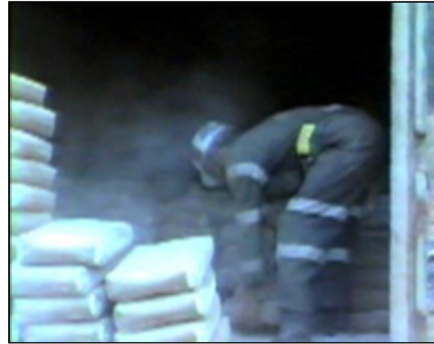
Lifting bags of rock dust from the storage area. Forceful exertions occur when lifting the bags and then when they are restacked for transportation. A bag of rock dust weighs 50 pounds.
