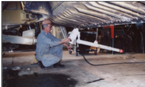
Heavy pneumatic wrench is attached to a counterbalance weight and supported by an overhead crane when changing the cutting edges on a blade.
