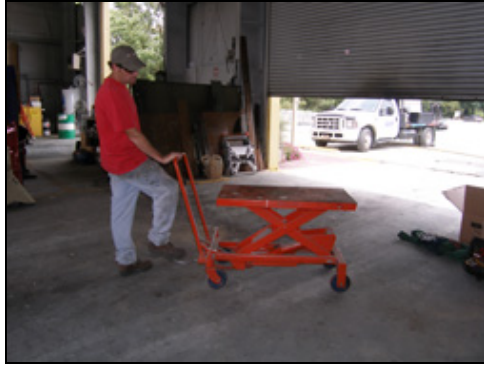
Scissors-lift table is used to position and work on parts when repairing equipment.
