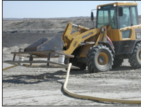
Tractor with a cable attachment is used to move dragline cable when positioning the dragline.
