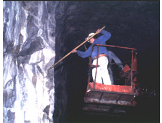
Hand scaling from a bucket. Miners must often use forceful exertions to remove loose rock from the rib.
