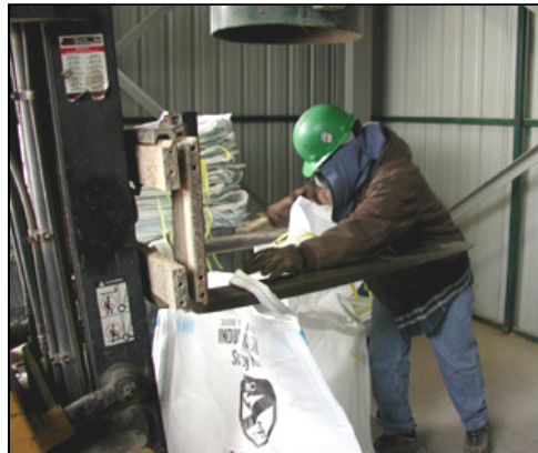
Workers sometimes use an excessive forward reach when placing an empty bulk bag on the forklift tines prior to filling the bag with product.
