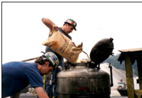
Workers lift bags of blasting materials and then support them while pouring the materials into the bin. Forceful exertions occur when lifting the bag into place and when holding the bag to pour the material.
