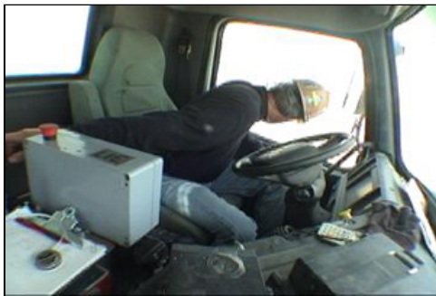
When aligning the prill auger above blast holes to dispense an explosive mixture, the miner turns his head to the left and looks over his shoulder while reaching backward with his right hand to operate the dispensing control.
