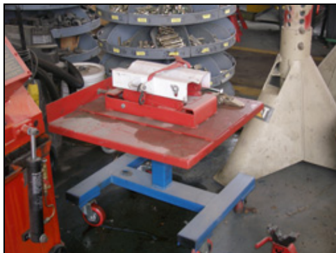
Small lifting table is used to hold parts when repairing equipment.
