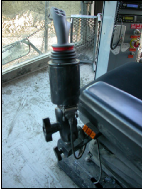
Adjustable joysticks can be placed close to the operator, which improves postures and eliminates reaching for the controls.
