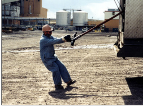
The greatest exertion usually occurs when starting to unwind the fuel hose from the storage reel.
