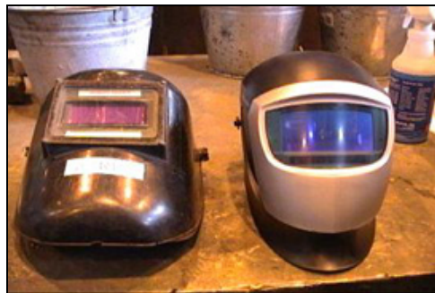
Light-weight welding helmets (right) reduce the effort needed to hold your head in a bent position while welding.
