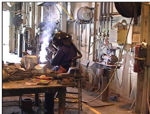
Often, the head is in a static position when looking downward at the weld joint. The neck and upper back muscles not only support the weight of the head when in this position, but also the weight of the welding helmet.
