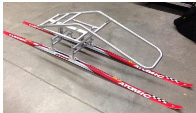
New Sitski with Articulating Lower Frame
