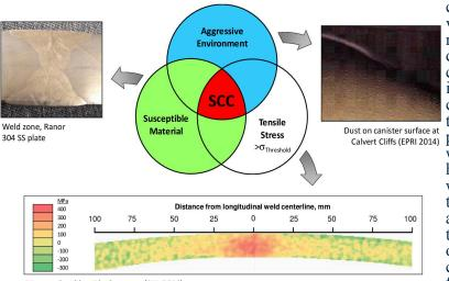
Measured weld residual stresses (SNL 2016)
