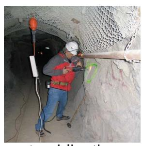
Seismic monitoring in a mine
