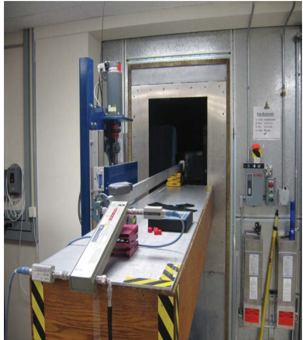
Figure 2. The waveguide with the standard gain horn used to transmit into the anechoic chamber. A dual directional coupler is used to measure power with two isolated power meters.
