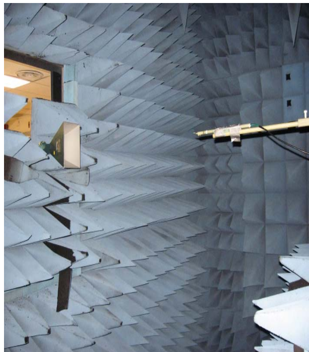
Figure 3. The 8 x 5 x 5 m 3 shielded anechoic chamber is used to calibrate probes from 500 MHz to 50 GHz.
