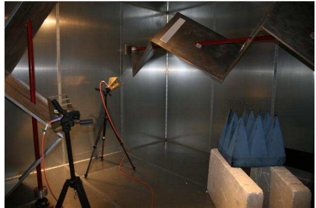
Figure 1 – Reverberation chamber used in the measurements with absorber in position 10.
