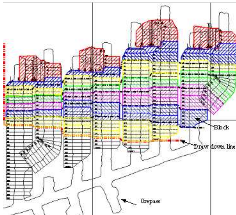
Figure 1.2. Machine placement MP849.29-30 consists of eight columns of production blocks. Notional drawdown lines pass through a “row” of blocks. The ore body is mapped onto an underlying network of production drifts, which connects to the ore pass.
