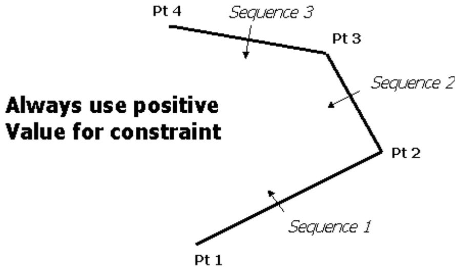
In the figure above, there are three line segments defining the capture zone. If there is more than one capture zone, then you would change the capture zone number on the line boundary dialog too. Again, the capture zones must be numbered starting with 1.
