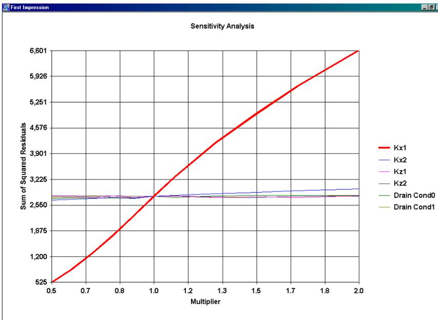
This curve shows that reducing  $K_{x1}$  by a factor of 0.5 would substantially reduce the sum of squared errors and therefore improve the quality of the calibration. Make that change now by selecting Props/Property Values/Database. After making the change, run the model one time to confirm the results and make another pass through the automatic sensitivity analysis. Do this a few times and see how much you can improve the calibration.
