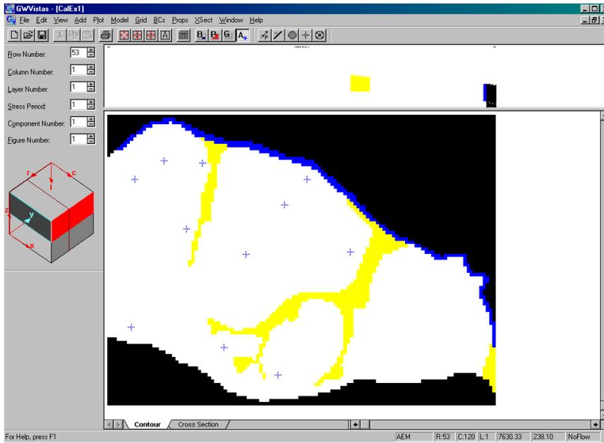
Run this model by either clicking the calculator button on the toolbar or by selecting **Model/MODFLOW/Create Datasets** and then selecting **Model/MODFLOW/Run MODFLOW**. Import heads when you are done and your screen should look like the following:
