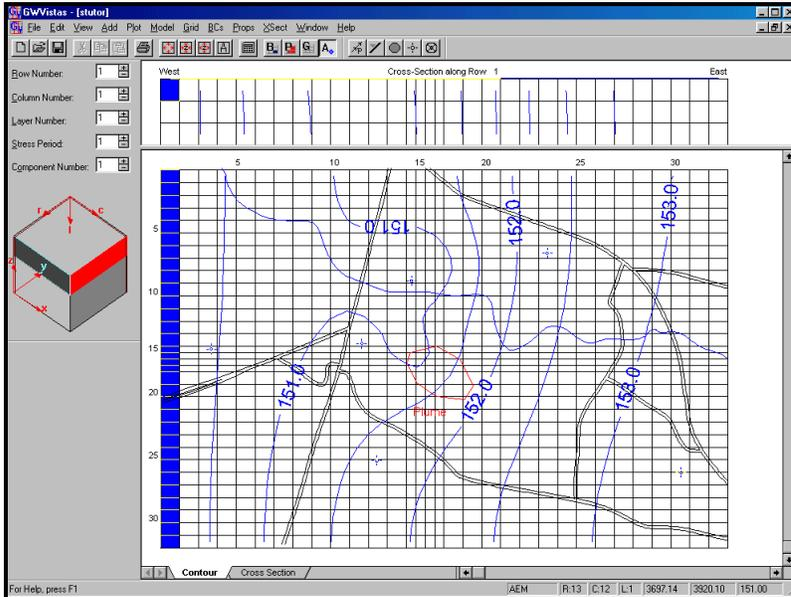
The contour map on your screen is the average of heads from the 100 realizations. To contour the standard deviation in head, select **Plot/What to Display.** Change the contoured variable from head to drawdown. Remember that drawdown in this case represents the standard deviation.
