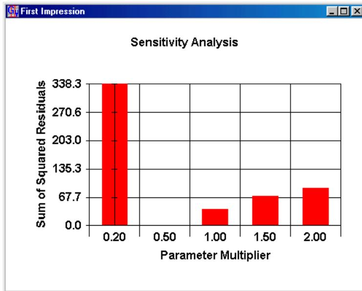
Note that a  $K_x$  value of half the current value gives a much better calibration because it has a lower sum of squared residuals than the current model (multiplier of 1.0 is the current value). If we were trying to achieve a better calibration in this model, we would probably want to lower the  $K$  value. We will explore this more in the next section.
