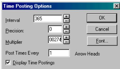
Now GV will redraw the traces with arrows spaced at equal time intervals instead of distance intervals. This is handy for looking at capture zones around wells for different time intervals.
