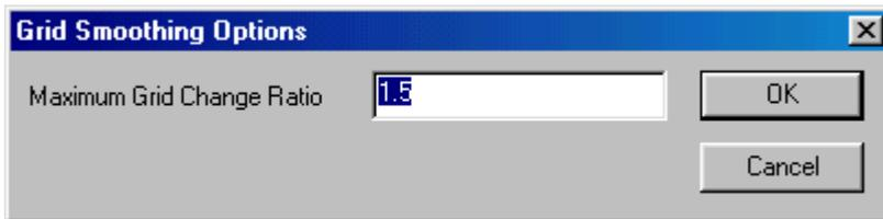
The grid smoothing option is very different from the one in Visual MODFLOW which some users may be familiar with. In Visual MODFLOW, the grid is smoothed but no rows or columns are added. This can result in a very different looking grid after smoothing. The approach used in GV tries to minimize the impact on grid spacings by adding rows or columns where necessary to achieve the maximum ratio.
