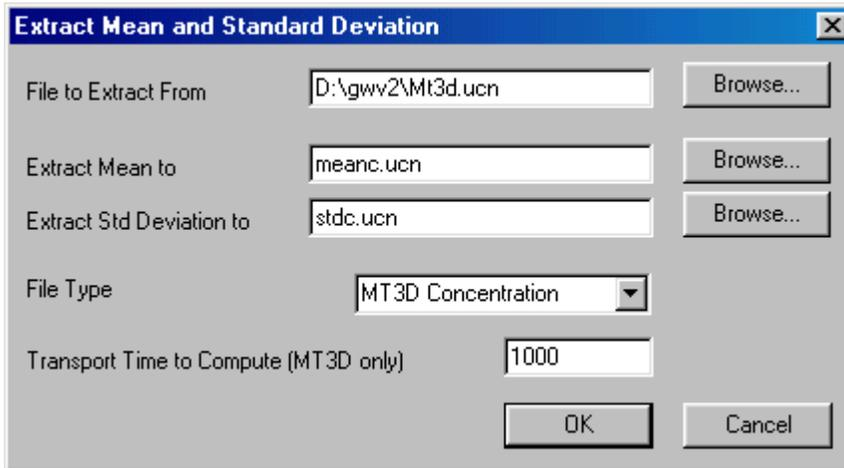
Be sure to specify the transport time of 1000 and that the file type is an *MT3D Concentration* file. You can now import the mean concentration and mean heads by selecting **Plot/Import Results**. The mean contaminant plume should look like the one shown below.
