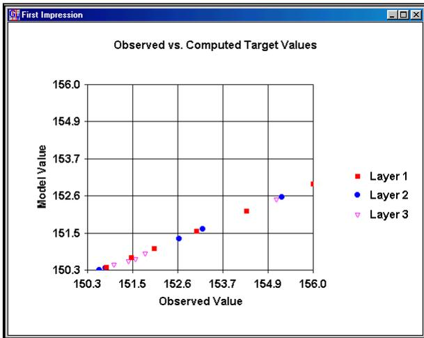
Ideally the plot shown above should be a straight line oriented at a 45-degree angle. This means that the observed value should equal the simulated value. In this example, the plot is a straight line but there is a strong bias such that higher heads are simulated too low.
