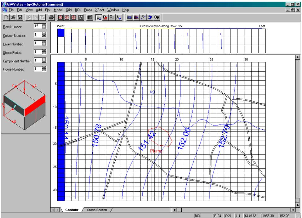
You can plot a hydrograph for the observation well you added by selecting **Plot->Hydrograph->Monitoring Well**. A dialog will show all of the observation wells in the model. In this case, there is only one. Click OK and your screen should look like the one below.
