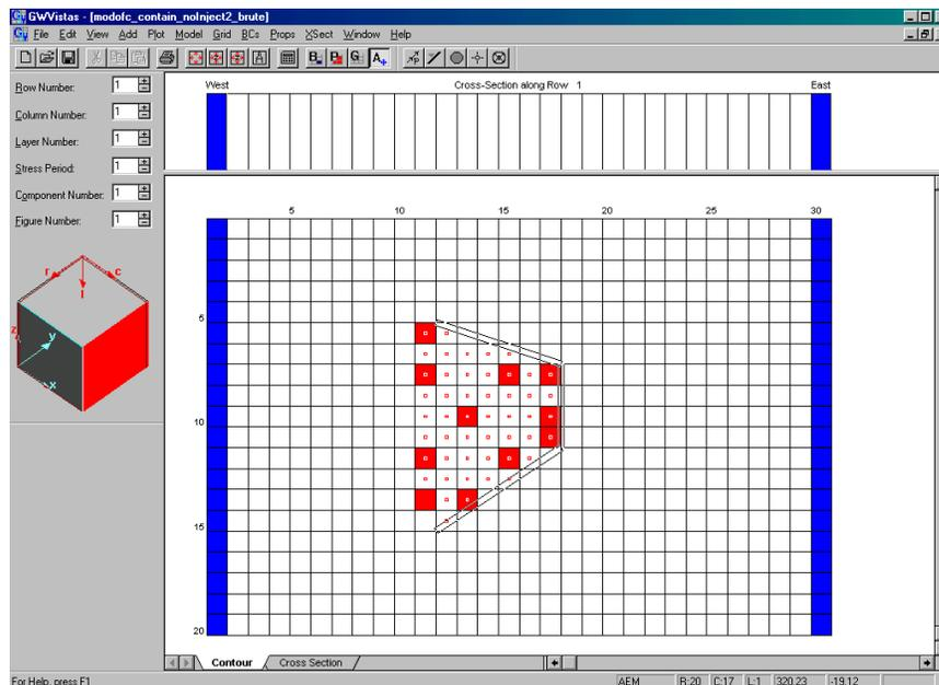
You can see the lines defining the capture zone and potential wells that are similar to the first MODOFC example. You also see a bunch of particles within the capture zone. These are for use with BF. The first thing to do is run one MODFLOW and one MODPATH simulation. These files form the basis for the next BF run. After running MODFLOW and MODPATH, your screen should look like the following:
