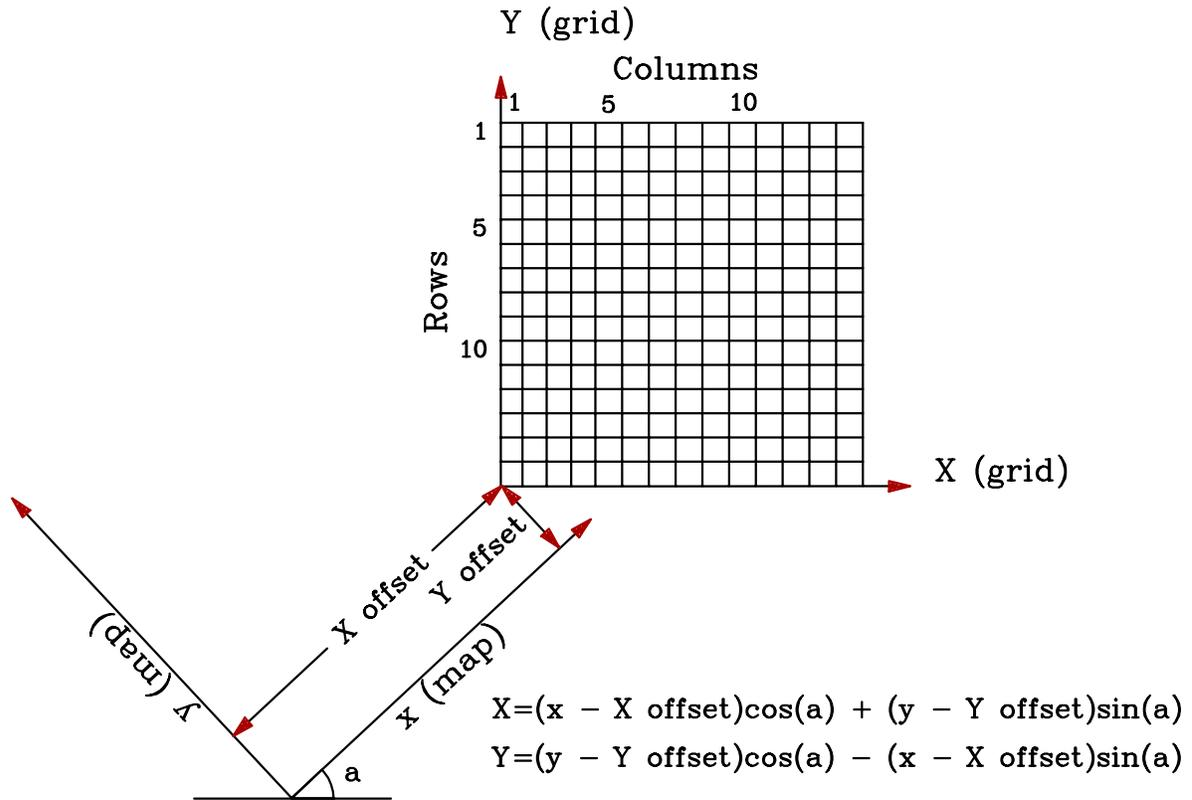
When digitized data, such as the base map or well coordinates, are used in the design of the model grid, they are first transformed (offset and rotated) to the new finite-difference grid coordinate system. This transformation is done automatically by GV, but you must be aware of the differences in coordinate systems when preparing the model dataset and base map.
