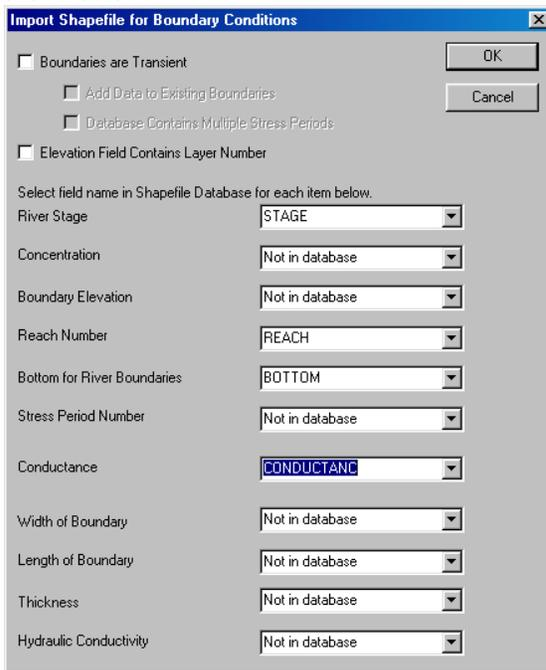
Since this is a one-layer model, we do not have layer information in the database. In this case, GV just puts the boundary conditions in the current layer. Now, your screen should look like the one below.
