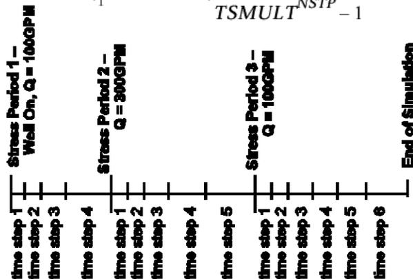
Create a transient flow model from the steady state model
