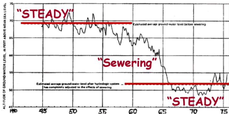
Suppose you wanted to simulate the impact of a proposed municipal water supply well that would go on line in 1962. In order to obtain a consistent set of starting values for initial conditions in 1962, it would be necessary to simulate the early equilibrium that prevailed until 1955, add the stress of the gradually reducing recharge in space through time until reaching 1957, then continue simulating the reductions in recharge along with the addition of the pumping well.
