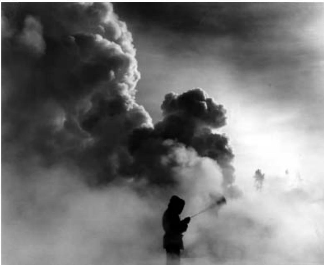
*Using a fist-sized chunk of dry ice fragments fastened to the end of a wire and swung in a circle overhead, a member of the 1962 Yellowstone Field Research Expedition (YFRE) seeds a supercooled cloud upwind of Old Faithful Geyser and along the road in front of the Old Faithful Inn.*
