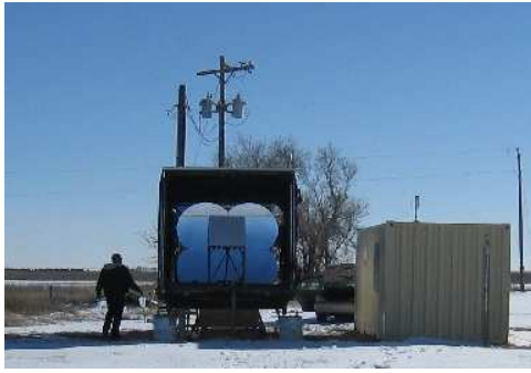
Figure 4: The remotely operated Atmospheric Monitoring Telescope (left) and its camera (right) with the central 4 columns instrumented. A rectangular UV transmitting filter (not shown) normally covers the camera surface.
