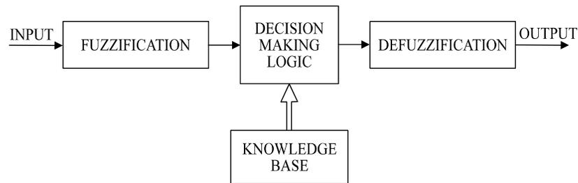
**Fig. 2** Fuzzy Controller Block Diagram
