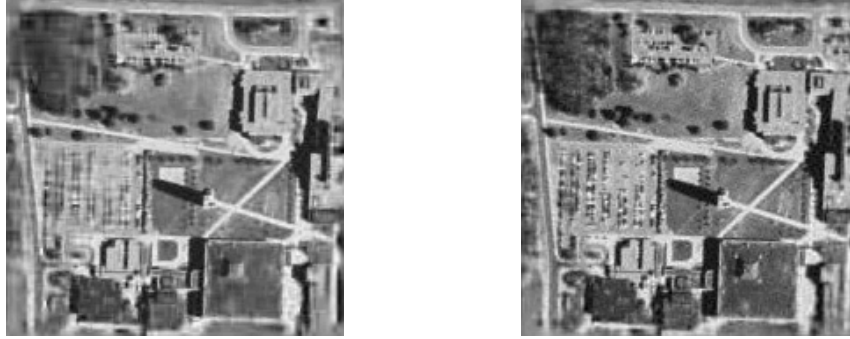
Fig. 7: Left: joint reconstruction using transform coding measurements with known camera positions, PSNR 22.8dB. Right: joint reconstruction using random measurements with known camera positions, PSNR 24.7dB.
