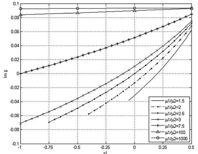
Fig. 4. Imaginary part of the singularity order  $\delta$  for the interface crack problem as a function of  $\nu_1$  (with  $\nu_2 = 0.30$ ) for  $1.5 \leq E_1/E_2 \leq 1000$ .
