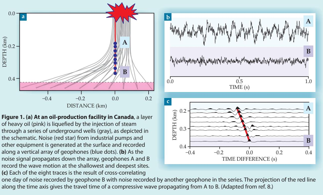
one obtains the same information that would be obtained in a controlled experiment using an impulsive source such as an explosion or earthquake to generate a pressure field. In the case of ambient noise, however, one speaks of a virtual source, not a real source.
