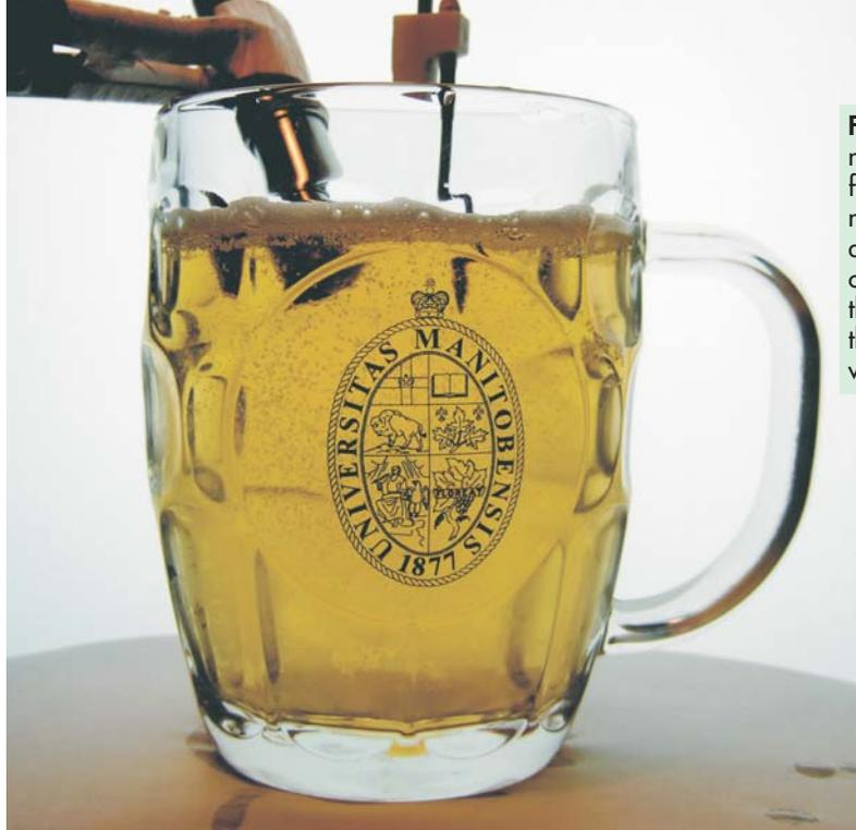
**Figure 6. Monitoring bubbles in beer.** A one-microsecond-long ultrasound pulse, at a center frequency of 1 MHz, is generated near the top of a mug of beer using an immersion transducer (top left) and detected with a needle-shaped hydrophone (top center). After many reflections off the mug's walls, the detected waves are sensitive to the evolution of the bubbles even when the bubble concentration is very low. (Photo courtesy of Valentin Leroy.)
