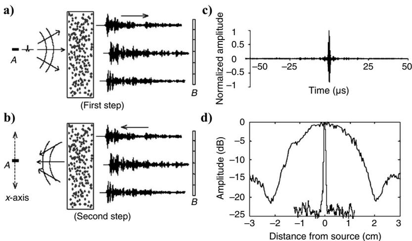
Figure 1. Time-reversed acoustics in a strongly scattering random medium (Derode et al., 1995; Fink, 2006). (a) The source at  $A$  emits a short pulse that propagates through the random medium. The scattered waves are recorded by the array at  $B$ . (b) The array at  $B$  emits the time-reversed signals, which, after back propagation through the random medium, focus at  $A$ . (c) The back-propagated response at  $A$ . (d) Beam profiles around  $A$ .
