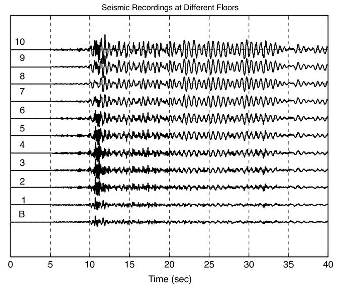
Fig. 4. Seismic recordings at the different floors (indicated as 1–10) with respect to basement motion (indicated as B or b).
