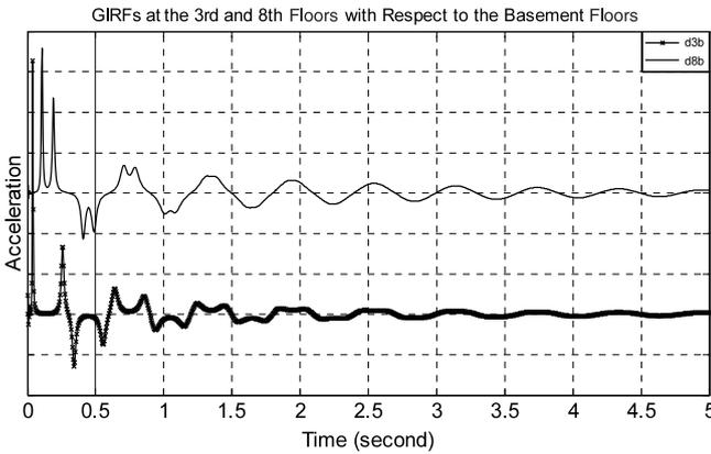
Fig. 6. GIRFs at the 3rd and 8th floors with respect to basement motion obtained based on Eq. (14) with selected parameters  $v_c = 322$  m/s,  $H_f = 48.2$  m,  $\gamma_c = 0.044$ .
