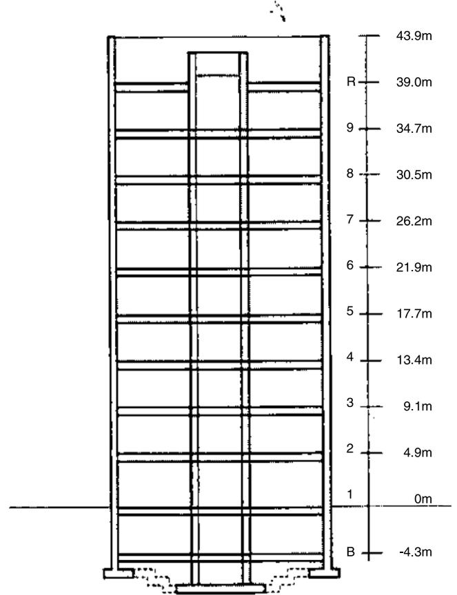
Fig. 3. Vertical cross section of the Millikan Library in the north–south direction.
