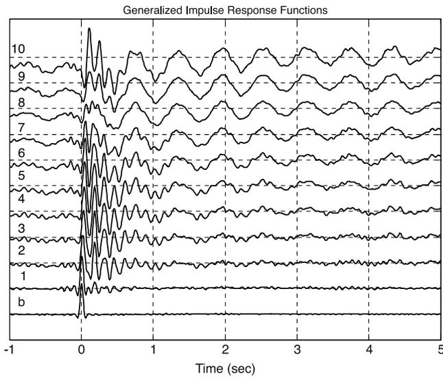
Fig. 5. GIRFs at the different floors (indicated as 1–10) with respect to basement motion (indicated as B or b).
