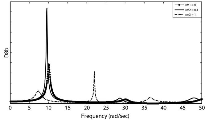
**Fig. 9.** GFRFs ( $D_{8bb}$ ) at the 8th floor of a 11-story building with respect to bottom motion with  $v_j = 300$  m/s,  $h_j = 4.25$  m,  $\gamma_{cj} = \gamma_j = 0.03$ ,  $r_{ij} = 1$  and  $r_{m11} = 0.5r_{m10}$ , for  $j = 1, 2, \dots, 11$ .
