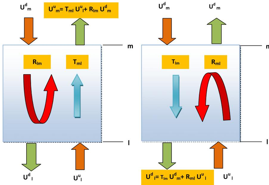
**Fig. 2.** Transmission and reflection coefficients  $T_{ml}$  and  $R_{lm}$  ((a) left) or  $T_{lm}$  and  $R_{ml}$  ((b) right) relate the out-going wave  $U_m^u$  (left) or  $U_l^d$  (right) and input waves  $U_m^d$  and  $U_l^u$  in building segment bounded by  $(z_l, z_m)$  or  $(l, m)$ .
