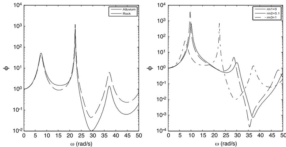
**Fig. 11.** Spectral density of acceleration at the 8th floor to ground acceleration spectral density with Kanai–Tajimi power spectra ( $G_0 = 1$ , site predominant frequency  $\omega_g$ , site damping  $\xi_g = 0.34$ ) with the same building parameters as Fig. 8. (a) (left)  $\omega_g = 18.4$  rad/s for alluvium and 27 rad/s for rock, and  $r_{mj} = 1$  and (b) (right)  $\omega_g = 18.4$  rad/s for alluvium and  $r_{mj} = 0, 0.1$  and 1.
