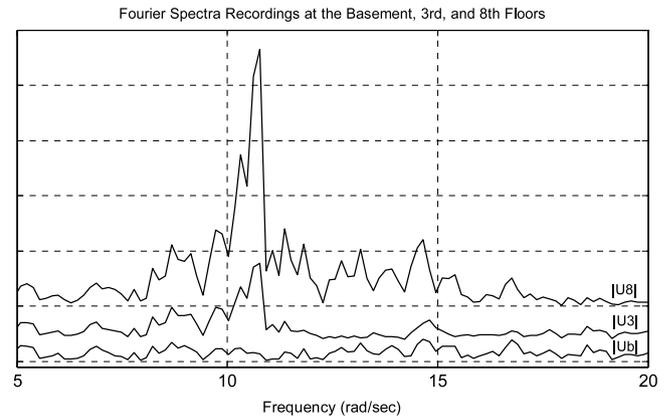
Fig. 8. Fourier spectra of seismic recordings at the basement, 3rd and 8th floors.
