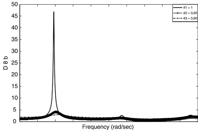
**Fig. 10.** GFRFs ( $D_{8b}$ ) at the 8th floor of a 11-story building with respect to bottom motion with  $v_j = 300$  m/s,  $h_j = 4.25$  m,  $\gamma_{cj} = \gamma_{ff} = 0.03$ ,  $r_{mj} = 0.1$  and  $r_{m11} = 0.5r_{m10}$ , for  $j = 1, 2, \dots, 11$ .
