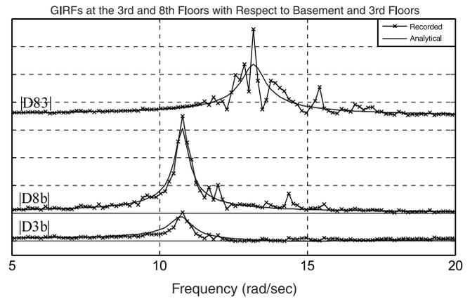
Fig. 7. Magnitudes of GFRF at the 3rd and 8th floors with respect to basement and 3rd floor motion obtained based on seismic recordings and theory in Eq. (14).
