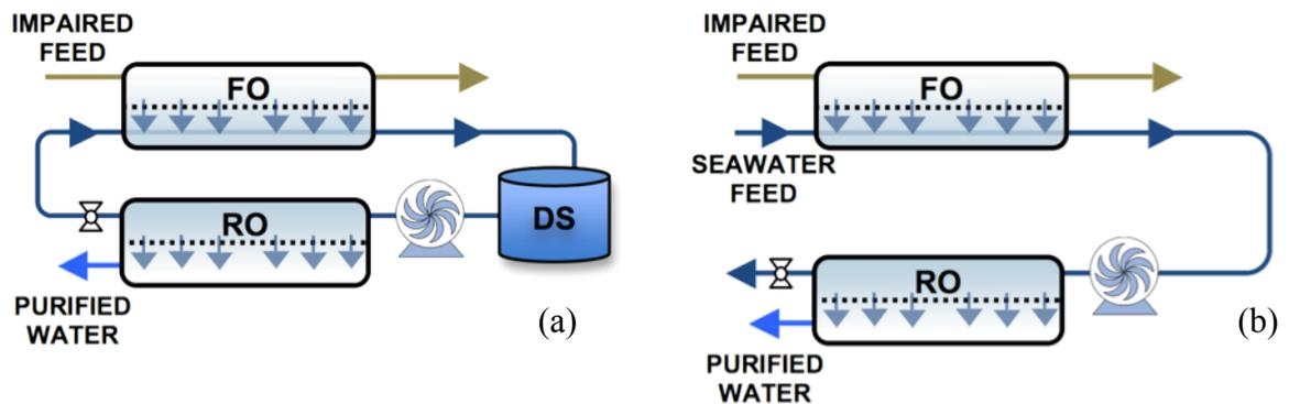
**Figure S1.** Two configuration of the hybrid FO-RO process: (a) closed loop DS in which the FO recovers water from an impaired stream and the RO reconcentrated the DS for reuse and simultaneously produces purified water, and (b) open loop DS in which the FO recovers water from an impaired stream that dilutes pretreated seawater on the way to a seawater reverse osmosis process.
