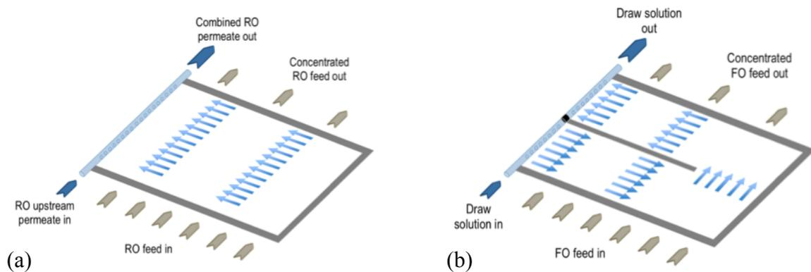
**Figure S2.** Flow patterns in a spiral wound module used for (a) RO and (b) modified for FO. The feed stream flows tangentially across the exterior of the rolled membrane envelope in both cases; however, the FO DS is forced to flow into the core tube and then through the interior of the membrane envelope before exiting the module.
