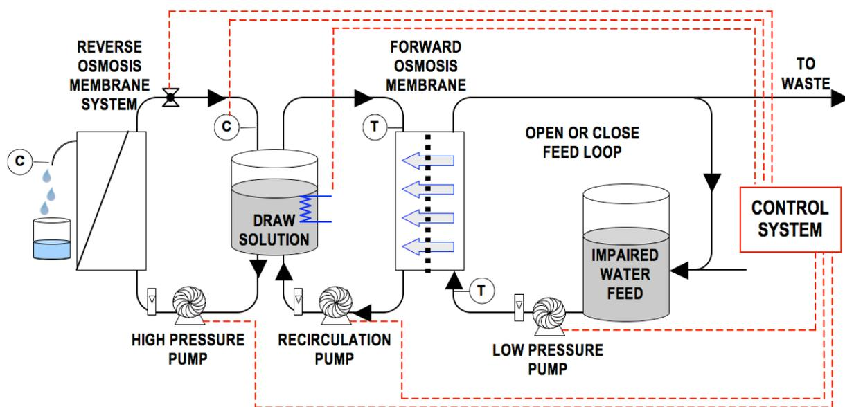
**Figure S3.** Schematics of the hybrid FO-RO pilot system.
