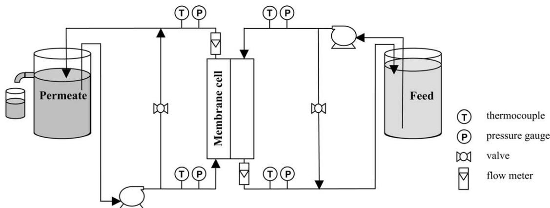
Fig. 1. Common DCMD apparatus.
