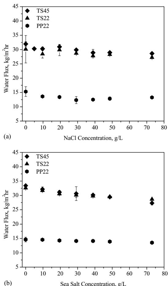
Fig. 10. Effect of (a) NaCl and (b) sea salt concentrations in the feed on flux in the DCMD/vacuum configuration. Feed and permeate temperatures are 40 and 20 °C, respectively; feed and permeate velocities are 1.4 m/s; and permeate absolute pressure is 69 kPa.
