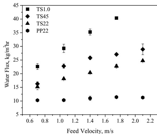
Fig. 4. Flux vs. feed velocity in traditional DCMD. Feed and permeate temperatures are 40 and 20 °C, respectively; feed salt concentration is 0.6 g/l NaCl.
