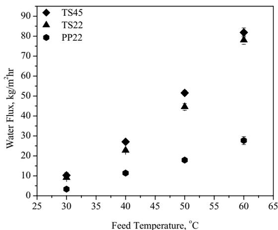
Fig. 5. Flux vs. feed temperature in traditional DCMD. Permeate temperature is 20°C; feed and permeate velocities are 1.75 m/s; feed salt concentration is 0.6 g/l NaCl.
