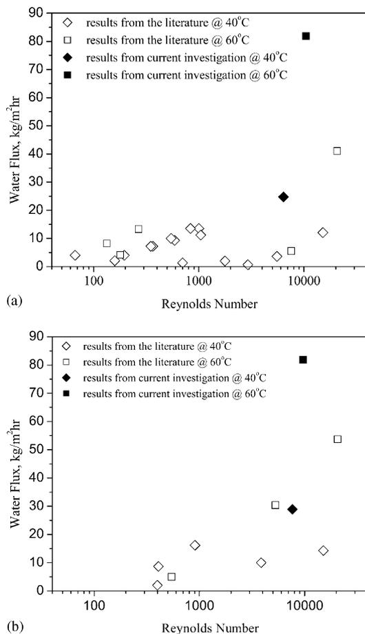
Fig. 7. Survey of previous MD studies with (a) 0.22  $\mu\text{m}$  and (b) 0.45  $\mu\text{m}$  hydrophobic membranes.
