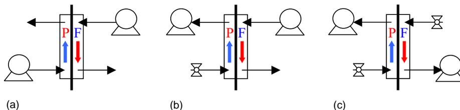
Fig. 3. DCMD configurations: (a) traditional, (b) vacuum on the permeate side, (c) vacuum on both sides.
