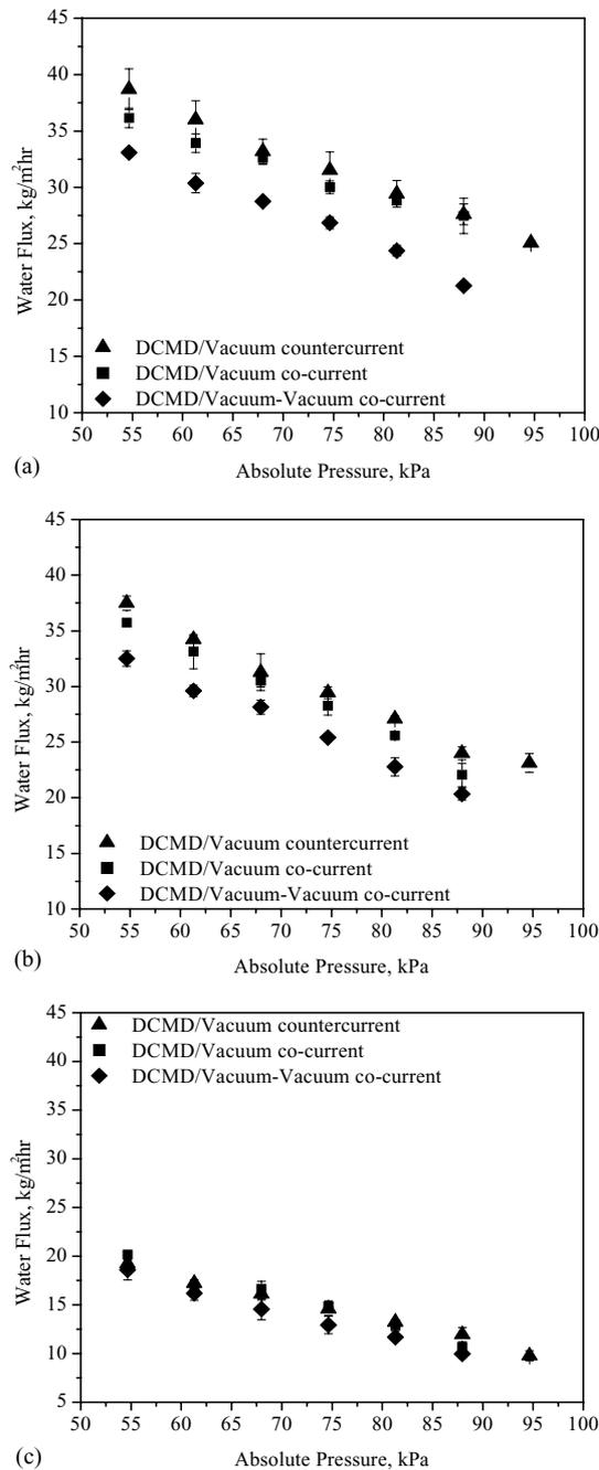
Fig. 11. Effect of flow pattern and feed-side vacuum on flux for the (a) TS45 (b) TS22 and (c) PP22 membranes. (◆) DCMD/vacuum in co-current mode, (■) DCMD/vacuum in countercurrent mode, and (▲) DCMD/vacuum–vacuum in co-current mode. Feed and permeate temperatures are 40 and 20 °C, respectively, and feed and permeate velocities are 1.4 m/s.
