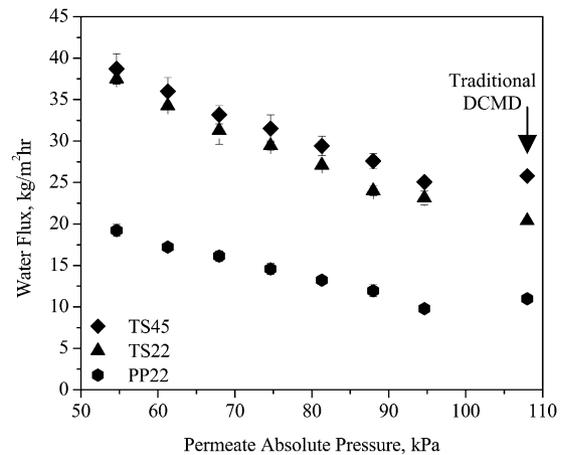
Fig. 9. Effect of permeate side vacuum on flux of water in the DCMD/vacuum configuration. Feed and permeate temperatures are 40 and 20 °C, respectively; feed and permeate velocities are 1.4 m/s; and feed salt concentration is 0.6 g/l NaCl. The reported pressure is at the inlet of the permeate side.
