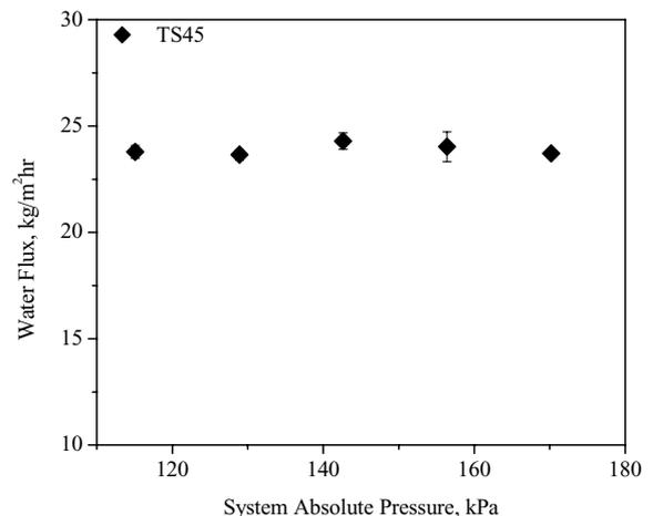
Fig. 6. Flux vs. system pressure in traditional DCMD. Feed and permeate temperatures are 40 and 20°C, respectively; feed and permeate velocities are 1.05 m/s, and feed salt concentration is 0.6 g/l NaCl.
