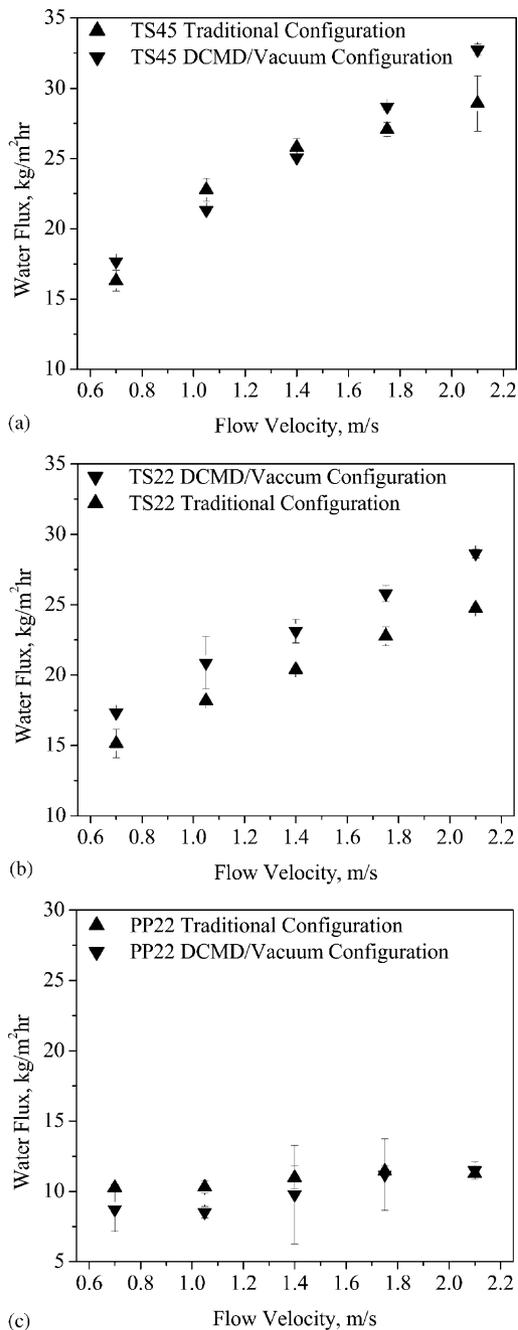
Fig. 8. Comparison of positive permeate pressure (traditional configuration) and negative permeate pressure (DCMD/vacuum configuration) on flux at various feed and permeate velocities for the (a) TS45 (b) TS22 and (c) PP22 membranes. Feed and permeate temperatures are 40 and 20 °C, respectively; absolute permeate pressures are 94 and 108 kPa; and feed salt concentration is 0.6 g/l NaCl.
