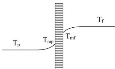
Fig. 2. Temperature polarization in MD.
