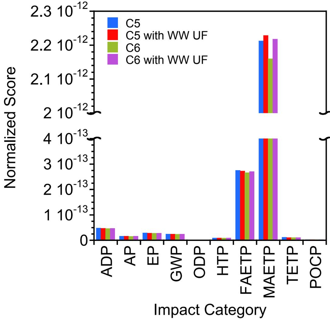
**Figure S3.** Normalized score of UF pretreatment of the ODN feed stream prior to the FO membranes across the ten impact categories of Scenarios C5 and C6 evaluated using data for the World in 1995 based on the CML 2 baseline 2000, V2.05. In all cases the ODN water recovery is 61% and the membrane packing density is 20 m<sup>2</sup>/module.
