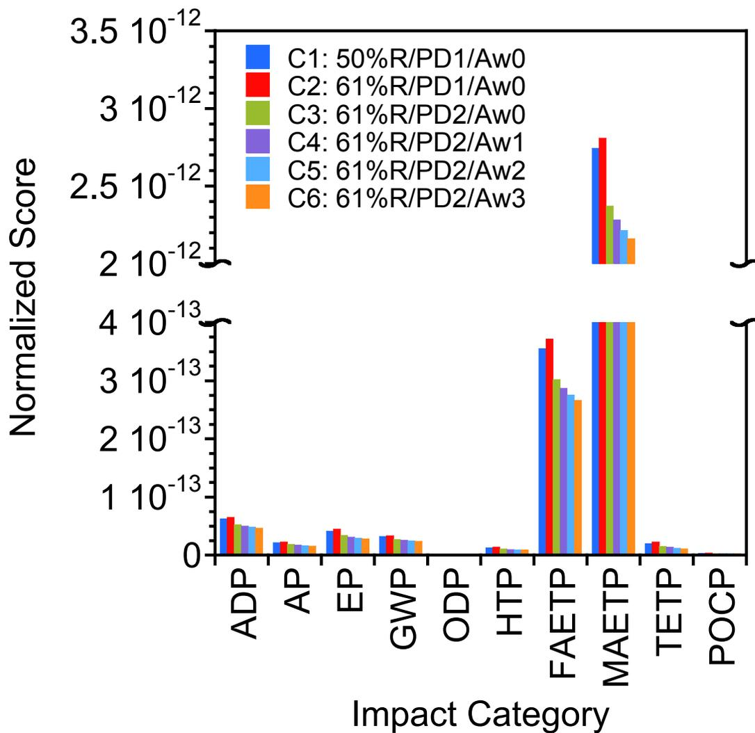
**Figure S2.** Normalized score of various improvements to the ODN membrane and module in Scenario C, evaluated using data for the World in 1995 based on the CML 2 baseline 2000, V2.05. %R represent percent ODN water recovery, PD1 represent packing density of 9.5 m<sup>2</sup>/module, PD2 represent 20 m<sup>2</sup>/module, and Aw represent the different FO membrane permeance coefficients.
