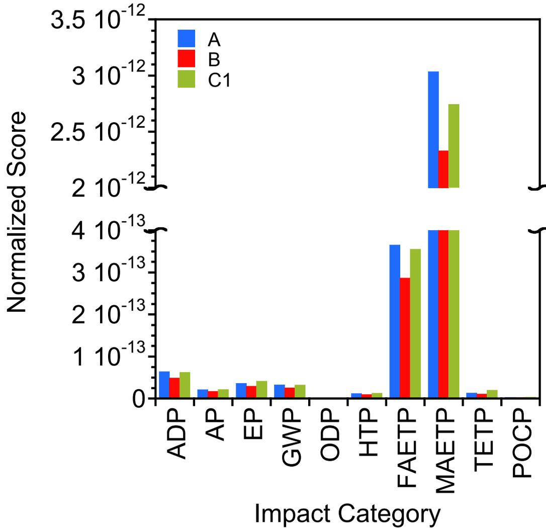
**Figure S1.** Normalized score of Scenarios A, B, and C1 evaluated using data for the World in 1995 based on the CML 2 baseline 2000, V2.05. Scenario C1 is for the ODN membrane with the baseline membrane  $A_{w0}$  value ( $0.36 \text{ L/m}^2 \cdot \text{h} \cdot \text{bar}$ ).
