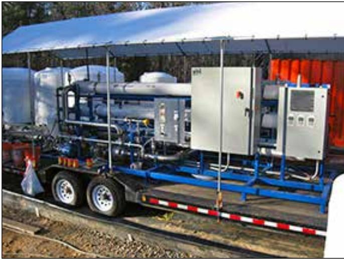
Company A's second generation of forward osmosis process A operates under constant influent draw solution concentration using a reverse osmosis membrane reconcentration system. The 8-in. spiral-wound forward osmosis elements are housed in membrane pressure vessels.
