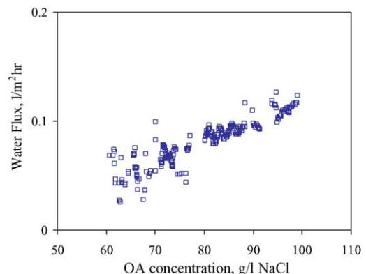
Fig. 3. Flux vs. OA concentration in the dual DO/OD process.
