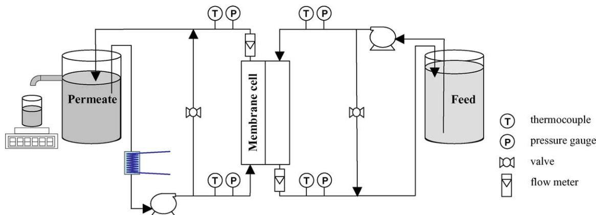
Fig. 6. Flow diagram of the bench-scale test unit.
