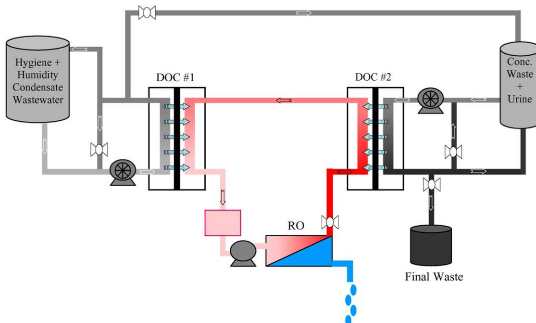
Fig. 1. Flow diagram of the NASA DOC wastewater treatment process.
