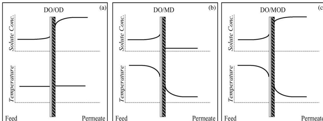
Fig. 5. Concentration and temperature profiles in (a) DO/OD, (b) DO/MD, and (c) DO/MOD.
