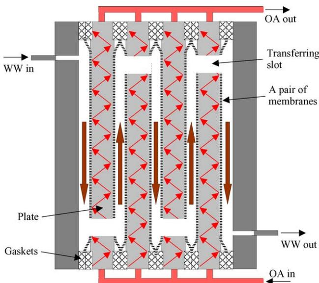
Fig. 4. Cross-section of the DOC#2 plate-and-frame design.
