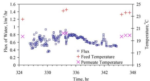
Fig. 9. A 24 h frame of bench-scale results in dual DO/MD membrane configuration.
