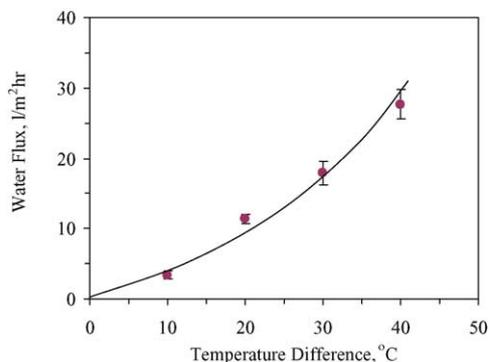
Fig. 7. Water flux as a function of temperature difference in MD with PP22 membrane.
