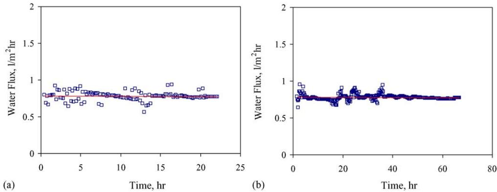
Fig. 8. Flux vs. time in the dual DO/MD process. For (a) urea solution feed and (b) concentrated synthetic feed.
