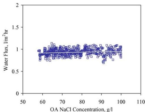
Fig. 10. Flux vs. OA concentration in the dual DO/MOD process.
