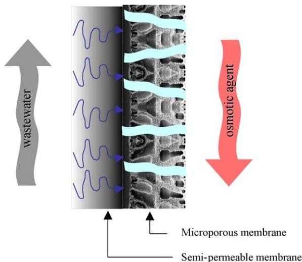
Fig. 2. Mass transport in the dual DO/OD membrane process in DOC#2.
