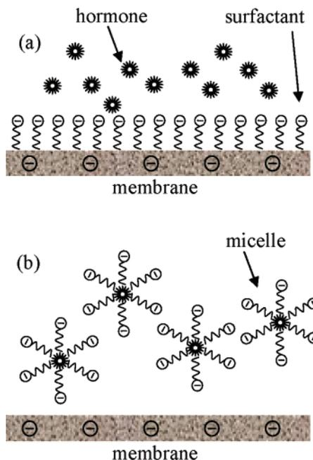
**FIGURE 6.** Schematic drawing of the proposed mechanisms by which anionic surfactants may facilitate increased FO hormone rejection (a) below and (b) above the CMC.
