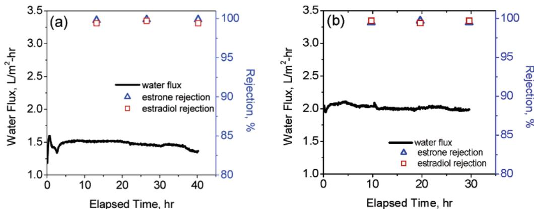
**FIGURE 4.** Water flux and estrone and estradiol rejection as a function of time during DCMD experiments. Feed solutions are either (a) wastewater stimulant containing urine and humidity condensate, or (b) DDW. Permeate samples were collected and analyzed for hormone rejection every time 2 L of water had permeated across the membrane.
