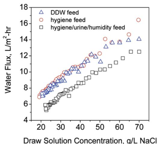
FIGURE 3. Water flux as a function of DS concentration during FO experiments. Feeds are DDW, wastewater containing only the hygiene component, or wastewater containing a mixture of hygiene, urine, and humidity condensate components.
