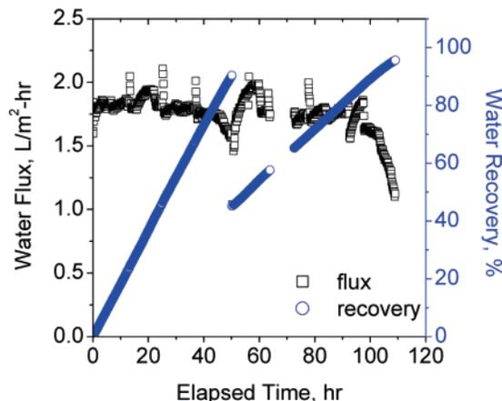
FIGURE 2. Water flux and recovery during a long-term semi-batch DCMD experiment with urine simulant as the feed solution. Temperature difference across the membrane is 20 °C and flowrates of both feed and permeate are 1.5 L/min.
