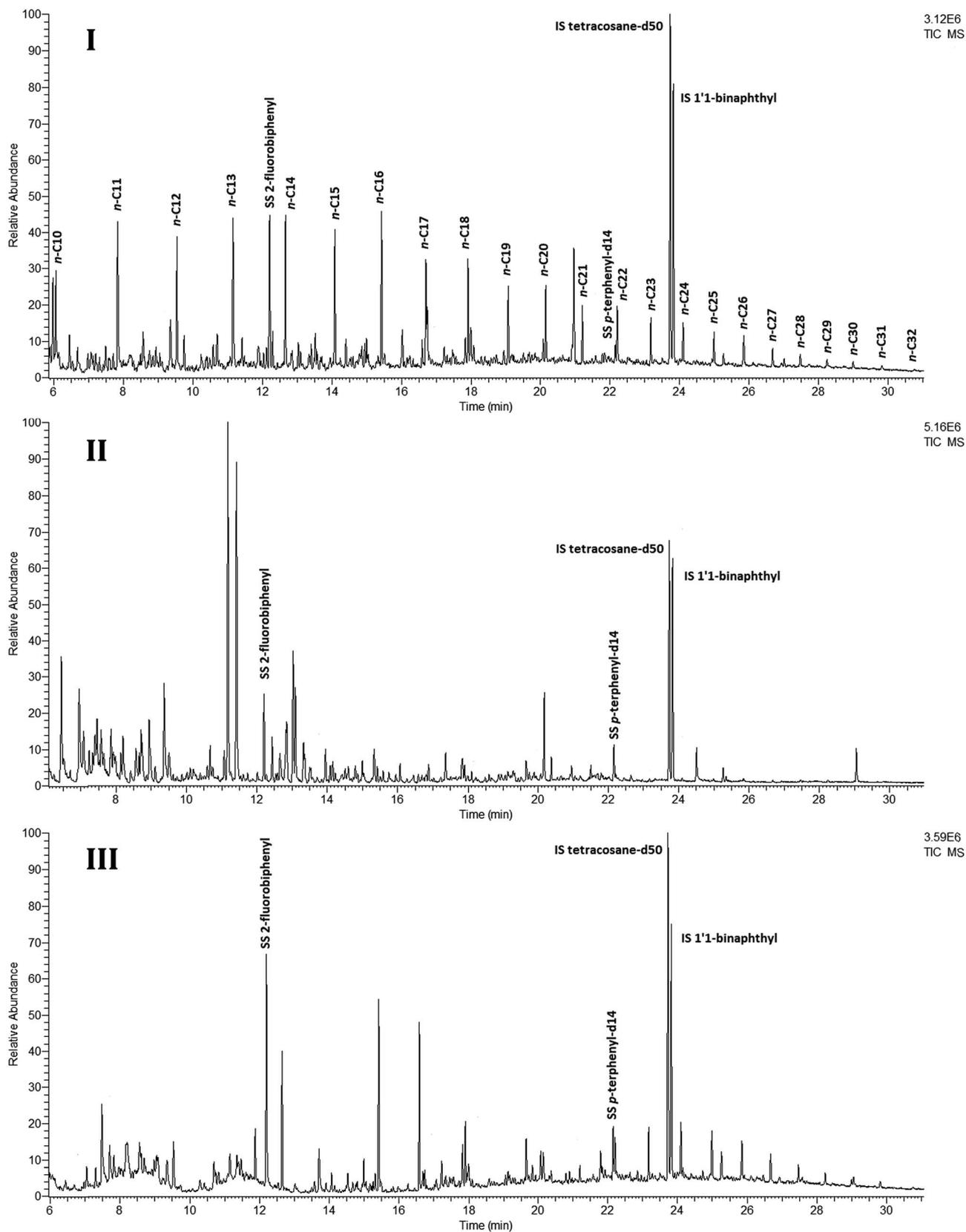
Fig. 2 Total ion chromatograms (TIC) of (I) produced water (1 mL sample enriched during solid phase extraction), (II) draw solution (400 mL sample enriched), and (III) RO permeate (400 mL sample enriched). Note that draw solution and RO permeate TIC are 400-times magnified compared to the produced water TIC. IS – internal standard, SS – surrogate standard.
