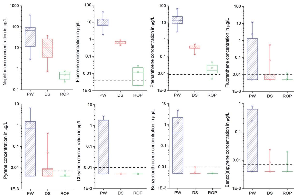
Fig. 5 Occurrence of eight selected PAH in the produced water feed (blue,  $n = 9$ ), draw solution (red,  $n = 9$ ), and RO permeate (green,  $n = 9$ ) of the pilot-scale hybrid treatment system. Note logarithmic scale on the y-axis. Black dashed line indicates method detection limit.
