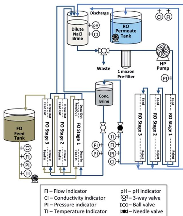
**Fig. 1** Simplified process flow diagram of the pilot-scale FO-RO hybrid treatment system (adapted from Hancock *et al.*).<sup>12</sup>
