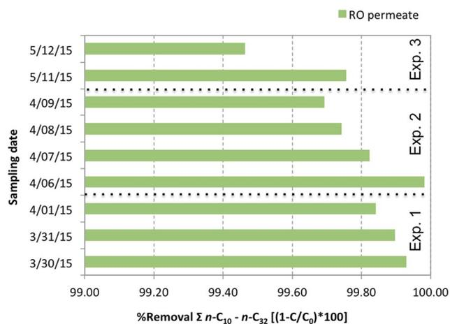
Fig. 4 Removal performance for *n*-alkanes (*n*-C<sub>10</sub>–*n*-C<sub>32</sub> range) during batch experiments 1, 2, and 3 by the pilot-scale FO–RO hybrid treatment system.
