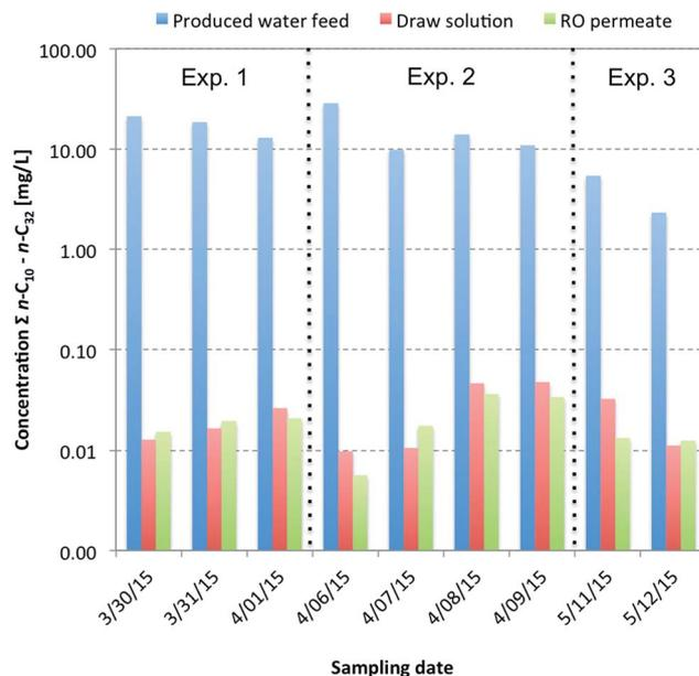
Fig. 3 Concentration of *n*-alkanes (sum of *n*-C<sub>10</sub> to *n*-C<sub>32</sub>) in the produced water feed, draw solution, and RO permeate of the pilot-scale hybrid treatment system during batch experiments 1, 2, and 3. Note logarithmic scale on the y-axis.
