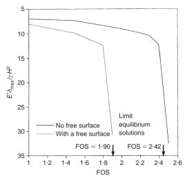
Fig. 18. Example 6: FOS versus dimensionless displacement
