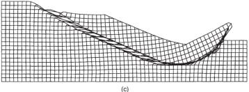
Fig. 8. Example 3: Deformed meshes at failure corresponding to the unconverged solution for three different values of  $c_{u2}/c_{u1}$  (a)  $c_{u2}/c_{u1} = 1.0$ ; (b)  $c_{u2}/c_{u1} = 0.6$ ; (c)  $c_{u2}/c_{u1} = 0.2$
