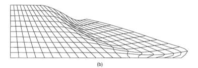
Fig. 4. Example 1: Deformed mesh plots corresponding to the unconverged solution with FOS = 1.4: (a) nodal displacement vectors; (b) deformed mesh
