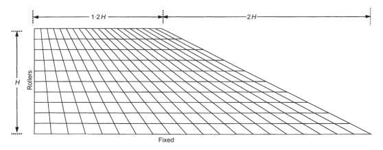
Fig. 1. Example 1: Mesh for a homogeneous slope with a slope angle of 26.57° (2:1),  $\phi' = 20^\circ$ ,  $c'/\gamma H = 0.05$
