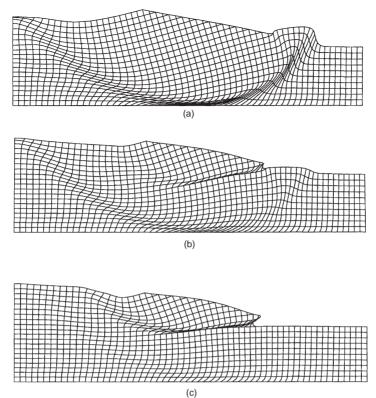
Fig. 11. Example 4: Deformed meshes at failure corresponding to the unconverged solution for three different values of  $c_{u2}/c_{u1}$ : (a)  $c_{u2}/c_{u1} = 0.6$ ; (b)  $c_{u2}/c_{u1} = 1.5$ ; (c)  $c_{u2}/c_{u1} = 2.0$
