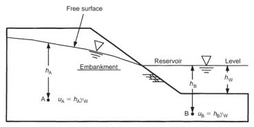
Fig. 12. Slope with free surface and reservoir loading
