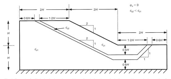
Fig. 6. Example 3: Undrained clay slope with a foundation layer including a thin weak layer (D = 2,  $c_{u1}/\gamma H = 0.25$ )
