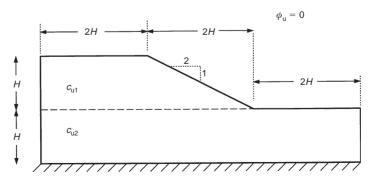
Fig. 9. Example 4: Undrained clay slope with a weak foundation layer  $(D = 2, c_{u1}/\gamma H = 0.25)$
