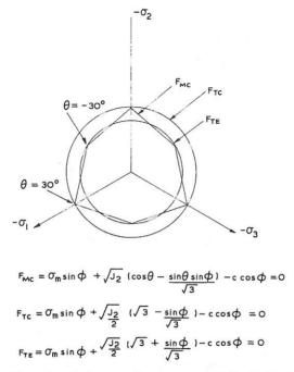
Figure 1. Surfaces used at corners of Mohr-Coulomb
