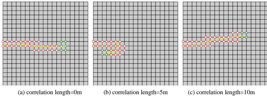
**Figure 6.** Fracture propagation pattern within random formations
