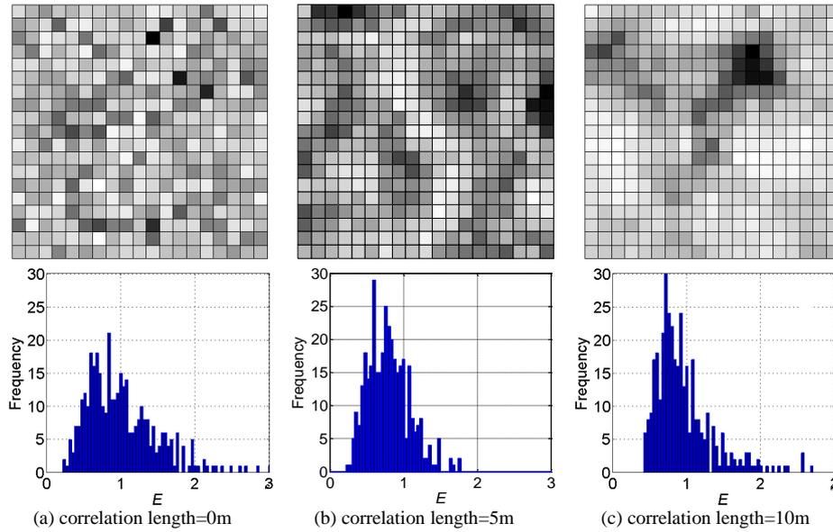
**Figure 4.** Random field examples and histograms of Young's modulus with different correlation lengths (mean=1MPa, standard deviation=0.5MPa)
