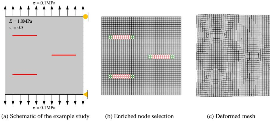
**Figure 3.** An example study using XFEM and COMSOL
