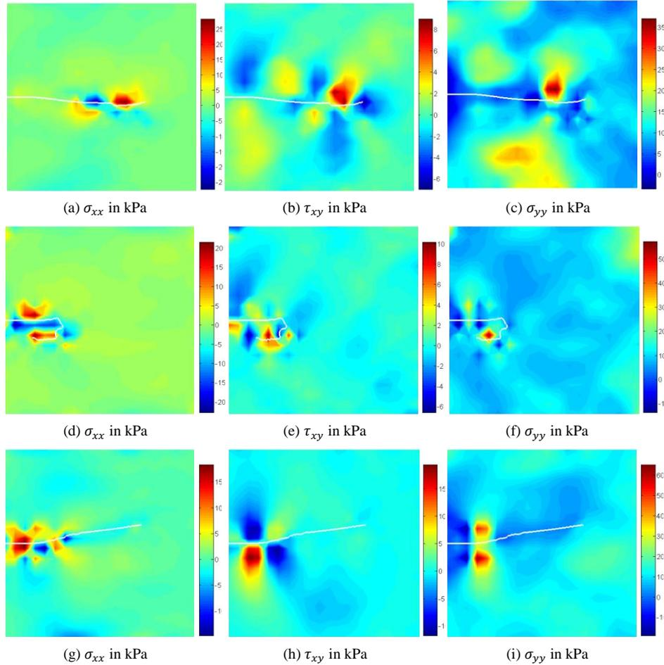
**Figure 7.** Stress contours (in kPa) within random fields of different correlation lengths (correlation length=0m for Figures 7(a)-7(c), correlation length=5m for Figures 7(d)-7(f), and correlation length=10m for Figures 7(g)-7(i))
