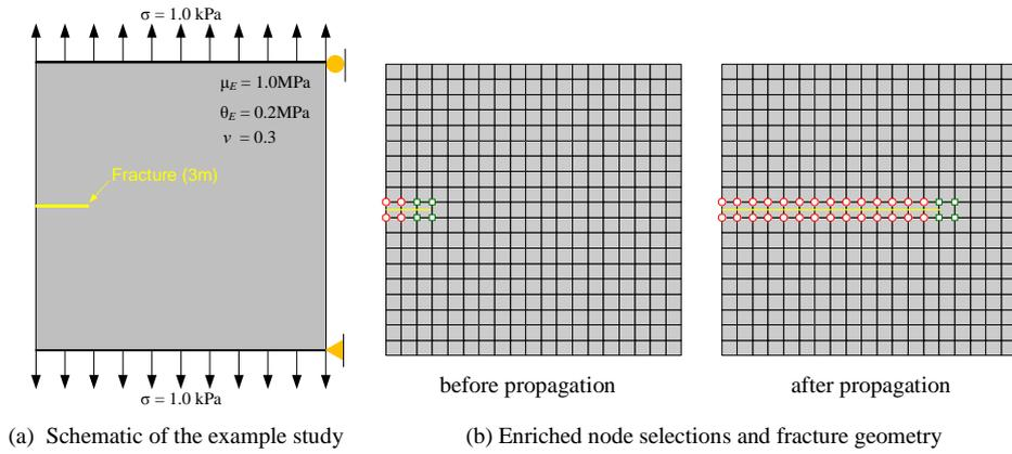
**Figure 5.** An example study using XRFEM
