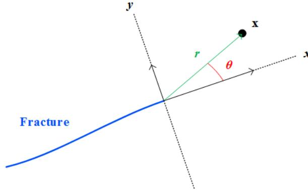
**Figure 2.** Fracture tip polar coordinates,  $r$  and  $\theta$  (Youn and Griffiths 2014)
