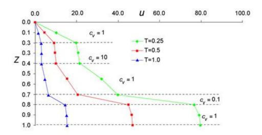
Figure 3: Excess Pore Pressure Distribution at Different Time Factors for Layered 1-D Consolidation
