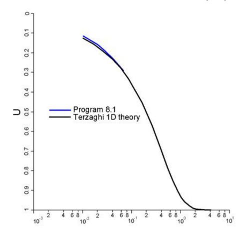
Figure 2: Computed and Exact Plots U vs. T For Homogeneous Case
