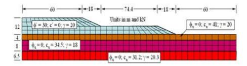
Figure 4: FE Geometry and Soil Properties Assigned to James Bay Dike
