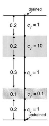
Figure 1: 1-D FE Mesh for Consolidation Analysis
