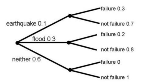
Figure 1. A simple event tree showing conditional probabilities that might lead to failure of an embankment.
