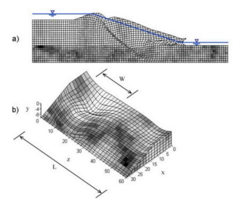
Figure 3. Typical RFEM simulations of slopes showing failure mechanisms "seeking out" paths through the weakest soils. a) 2D simulation of a tailings dam showing the development of two different failure mechanisms. b) 3D simulation of a long dam or levee showing a localized failure mechanism due to a zone of weaker soil.
