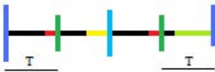
Fig. 3. Demonstration of Assumptions. Each interval T is constant, but the amount of "useful" work done in an interval changes (shown in black). The other colors show the respective amounts of time spent checkpointing for the checkpoint after them.
