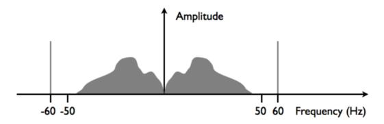
The spikes in the spectrum at  $\pm 60$  Hz are caused by power line noise. Now assume that this signal is sampled uniformly with interval T = 0.01 s to obtain a sequence x[n].
