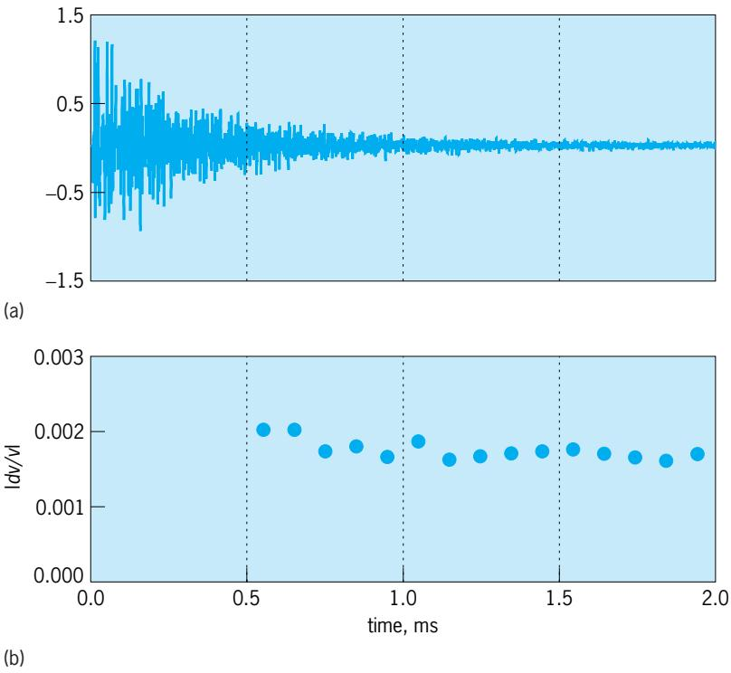
**Fig. 2. Measuring velocity change.** (a) Ultrasound waves were recorded in a small granite sample. (b) The relative velocity change for a 5°C (9°F) increase in temperature as a function of the center time of each time window was used to measure the velocity change.
