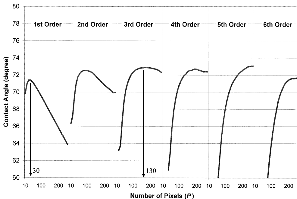
Fig. 10. Average contact angle for several polynomials of different order versus number of pixels. Each of the sections between the vertical gridlines represents a different polynomial (first-order to sixth-order); and the horizontal axis shows the number of pixels (10, 20, ..., 260) used in the fitting procedure.
